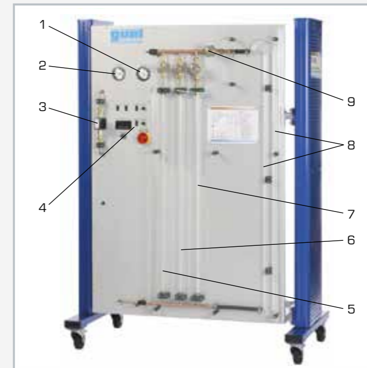
1 manometer delivery side, 2 manometer intake side, 3 flow meter, 4 display and control elements, 5 rising pipe Ø 6mm, 6 rising pipe Ø 10mm, 7 rising pipe Ø 14,4mm, 8 double rising pipe, 9 valve for rising pipe selection
