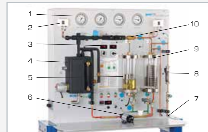
1 manometer, 2 pressure switch, 3 displays and controls, 4 vapour generator, 5 evaporator, 6 pump, 7 cooling water connections, 8 flow meter, 9 condenser, 10 vapour jet compressor
