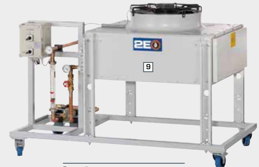
Dry cooling tower
