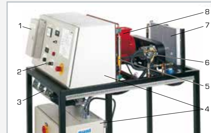
1 box with fault buttons, 2 ignition key, 3 air cooler with three-stage fan, 4 switch cabinet, 5 flow meter, 6 compressor, 7 condenser with fan, 8 electric motor
