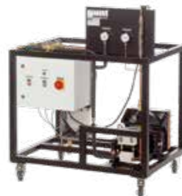
WL 312.12 Condensing unit
