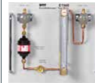
Sight glass with filter/drier and flow meter
