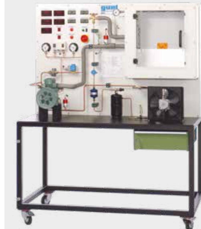
ET 165 Refrigeration system with open compressor
