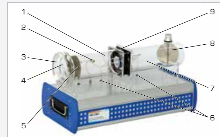
1 guide plates for flow guidance, 2 measuring point for temperature, 3 intake nozzle at intake pipe, 4 measuring point for pressure (to determine the flow rate), 5 flow straightener, 6 measuring points for pressure, 7 delivery pipe, 8 throttle valve, 9 axial fan
