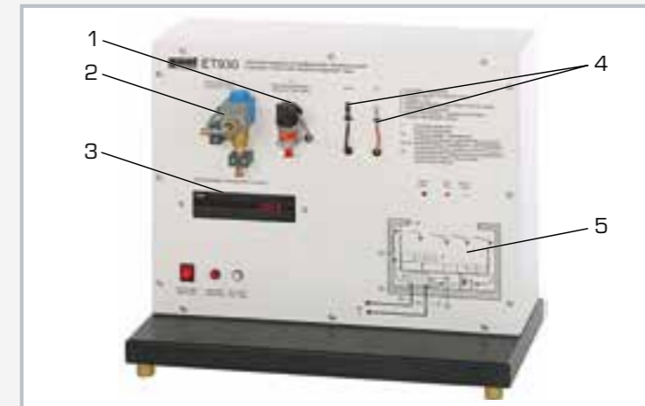
1 pressure sensor, 2 electronic expansion valve, 3 display of the refrigeration controller, 4 temperature sensor, 5 diagram of the simulated freezer
