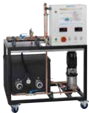
WL 312.10 Hot water generator
