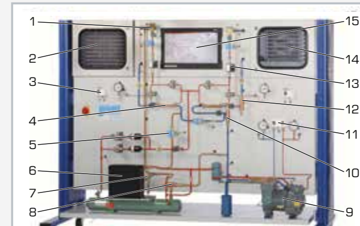
1 expansion valve, 2 freezing chamber, 3 thermostat, 4 heat exchanger, 5 solenoid valve, 6 condenser, 7 condensation pressure controller, 8 capacity controller, 9 compressor, 10 start-up controller, 11 pressure switch, 12 evaporation pressure controller, 13 flow meter, 14 refrigeration chamber, 15 touch panel PC
