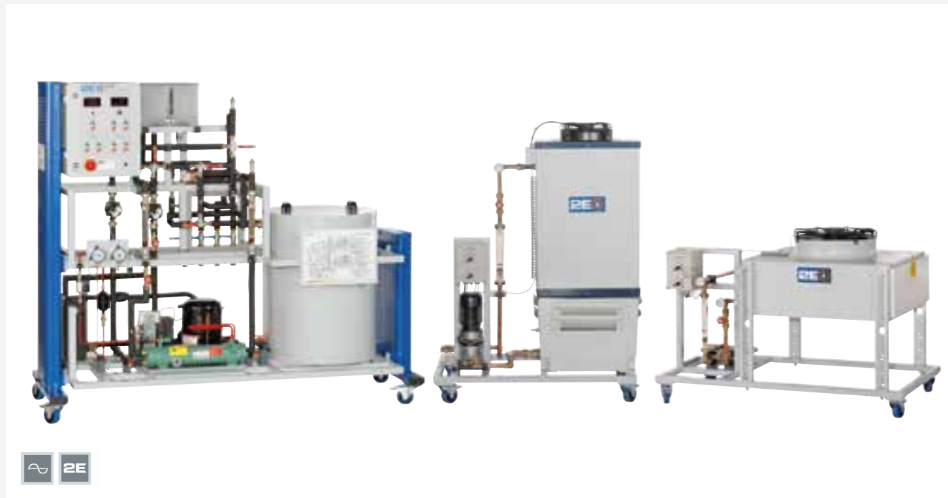
The illustration shows the trainer on the left, the wet cooling tower in the middle and the dry cooling tower on the right.
