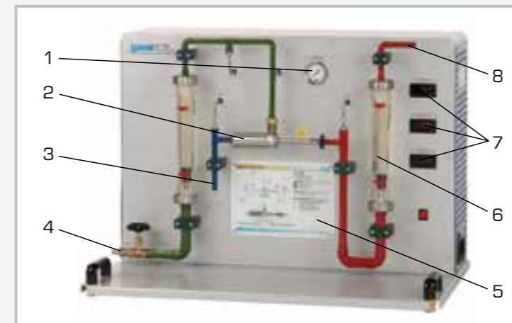
1 manometer, 2 vortex tube, 3 cold air outlet, 4 compressed air connection, 5 process schematic, 6 flow meter, 7 temperature displays, 8 hot air outlet
