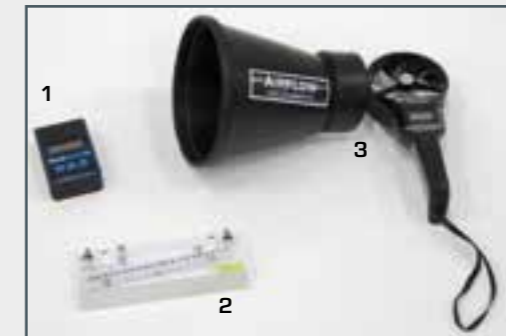
1 digital manometer, 2 inclined tube manometer, 3 anemometer
