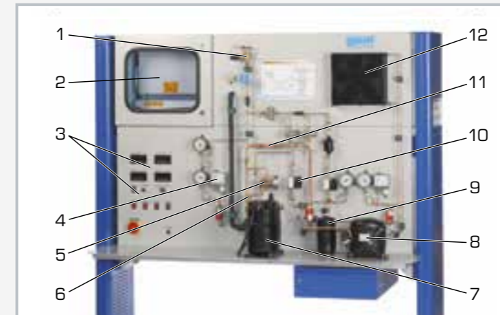
1 expansion valve, 2 refrigeration chamber, 3 displays and controls, 4 pressure switch, 5 injection valve, 6 injection cooler, 7 LP compressor, 8 HP compressor, 9 receiver, 10 flow meter, 11 heat exchanger, 12 condenser
