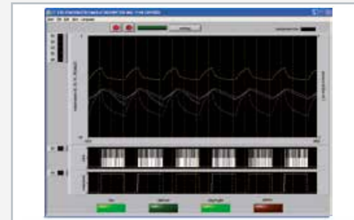
Screenshot of the simulation software: temperature graphs (top), switching states (bottom)
