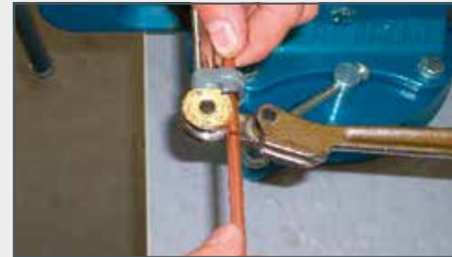
Inserting the pipe into the bending device
