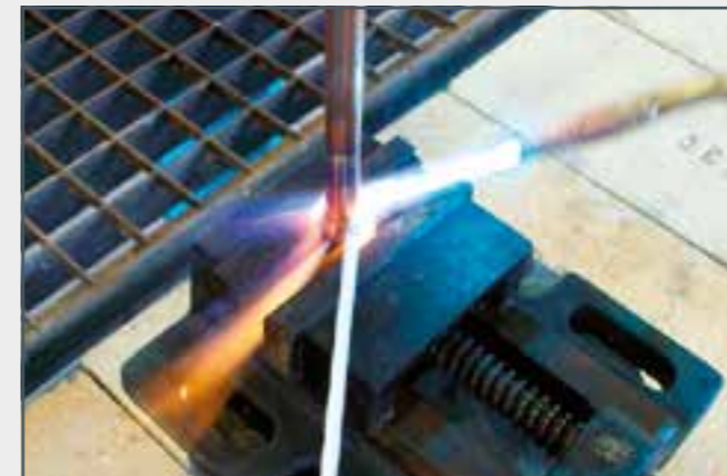
Heating the workpieces up to the soldering heat and melting of flux material and solder. By capillary effect solder automatically fills the soldering gap.
