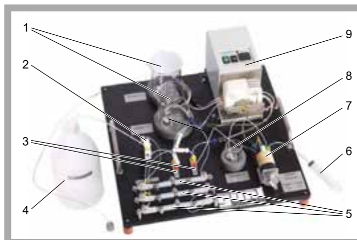
1 tanks for reagents A and B, 2 flow cell, 3 mixing chambers, 4 waste, 5 reaction loop, 6 injection syringe, 7 injection valve, 8 GOD, 9 multi-channel peristaltic pump
