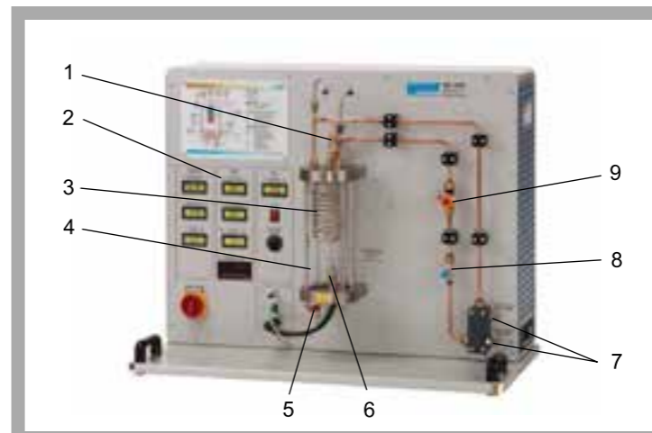
1 safety valve, 2 displays for temperature, flow rate and pressure, 3 condenser, 4 pressure vessel, 5 drain valve for the evaporating liquid, 6 heater, 7 cooling water connection, 8 valve for adjusting the cooling water, 9 cooling water flow rate sensor
