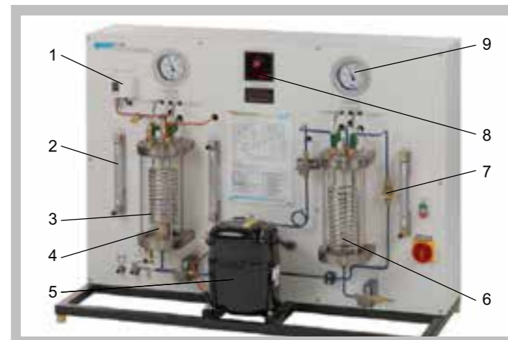
1 pressure switch, 2 flow meter, 3 condenser, 4 expansion valve, 5 compressor, 6 evaporator, 7 sight glass, 8 temperature display, 9 manometer
