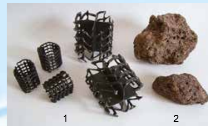
Carrier materials for biofilms: 1 artificial carrier material (plastic), 2 natural carrier material (e.g. extrusive rocks)
