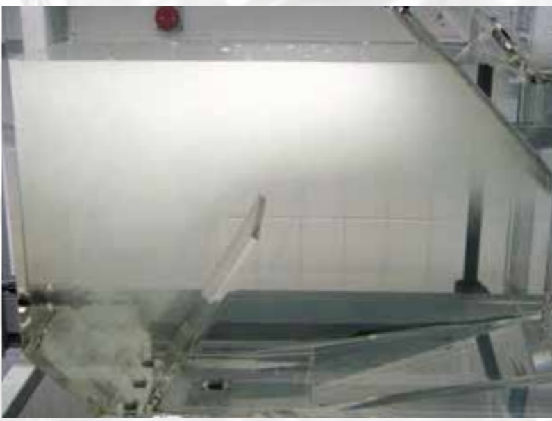
The recycle water enters the flotation tank: The sudden relief to atmospheric pressure causes the dissolved air to precipitate as a cloud of small bubbles.
