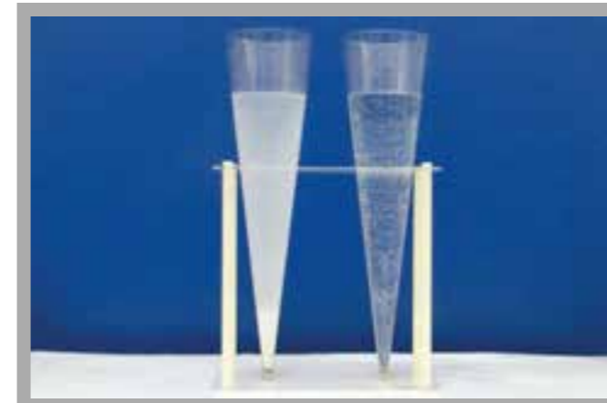
Determination of solid concentrations at sedimentation tank inlet and outlet by Imhoff cones
