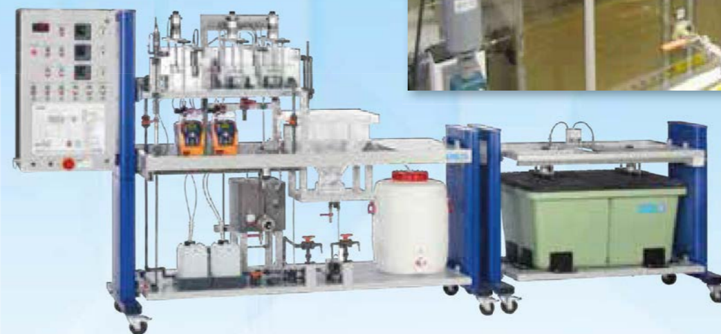
CE 705 Activated Sludge Process
