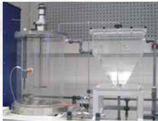
Stirred tank with secondary clarifier
