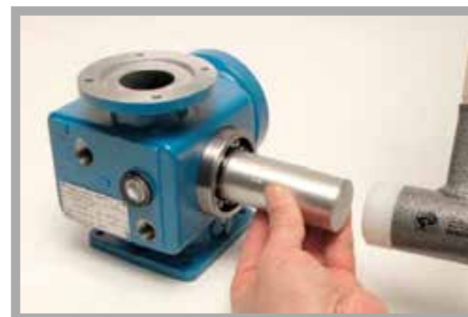
Assembly of the diaphragm pump: driving the eccentric into the housing (using a device)
