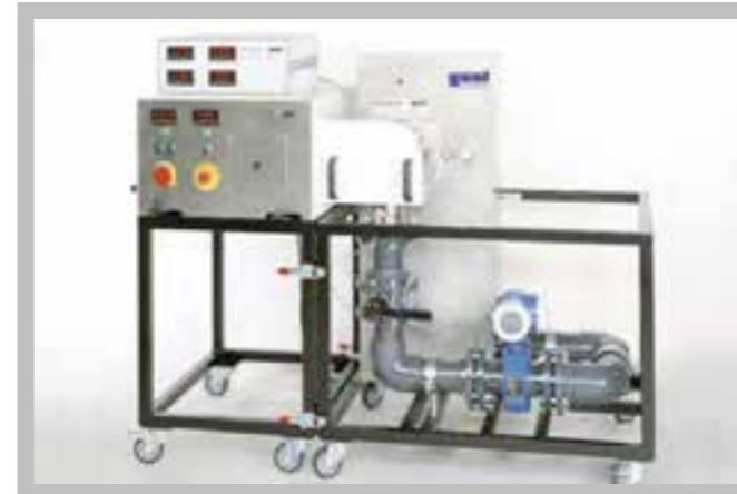
This picture shows a complete experimentation set-up: axial-flow pump HM 365.45 connected to the universal drive and brake unit HM 365
