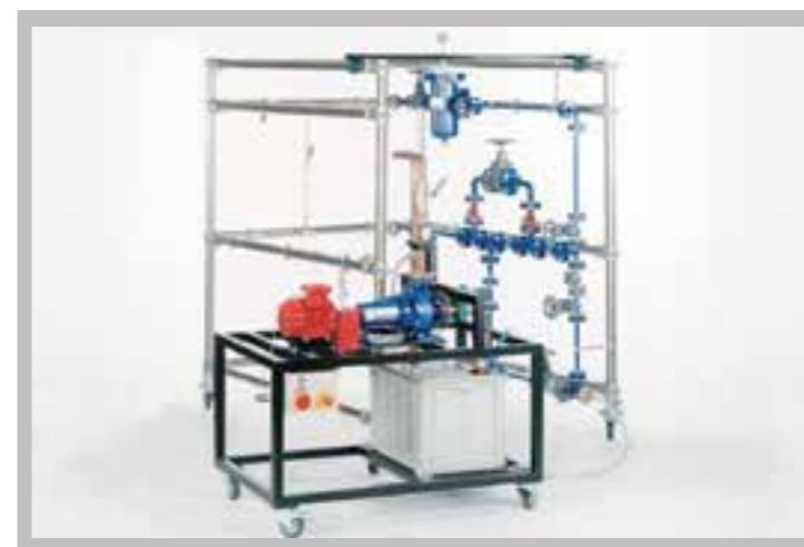
The picture shows HL 960 with a completed specimen installation. In the foreground: pump system HL 960.01.
