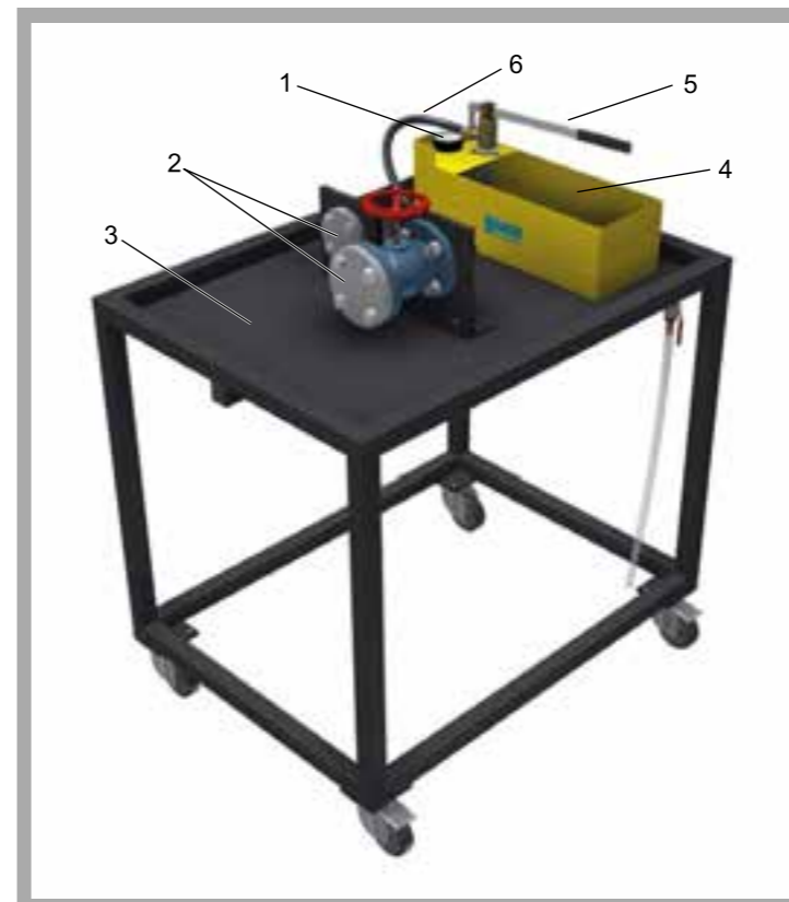
1 manometer, 2 mounting flanges with blank flange, 3 benchtop tray with drain, 4 pressure test pump with water tank, 5 hand lever, 6 hose
