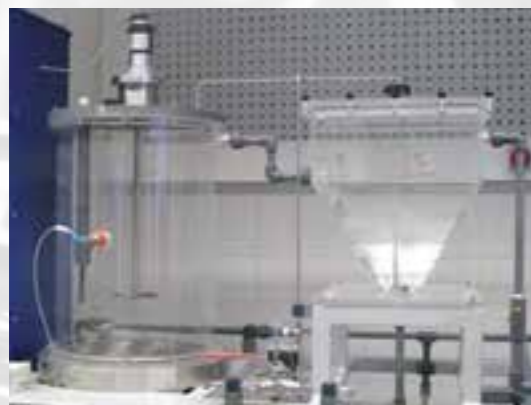
Stirred tank with secondary clarifier
