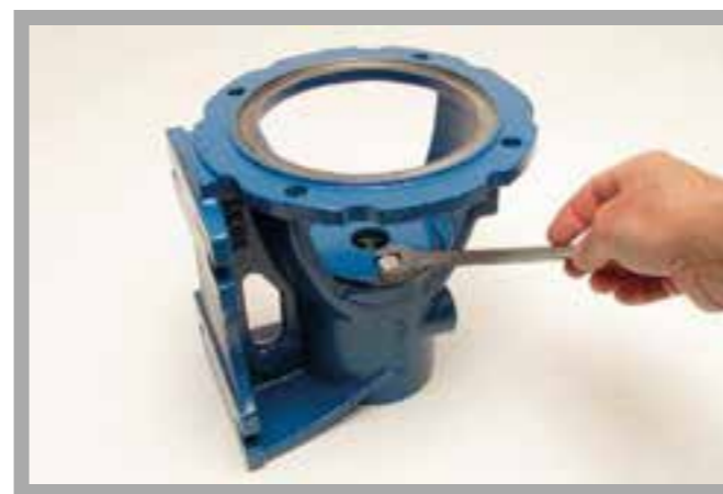
Assembly of the centrifugal pump: fixing of the bearing cover with screws
