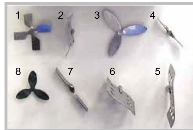
Stirring heads: 1,3,8 propeller stirring heads, 2,5,6 paddle stirring heads, 4,7 propeller stirring heads, angled
