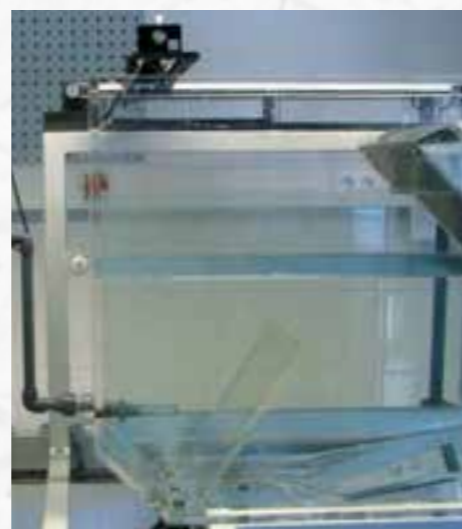
2 Flotation tank with scraper
