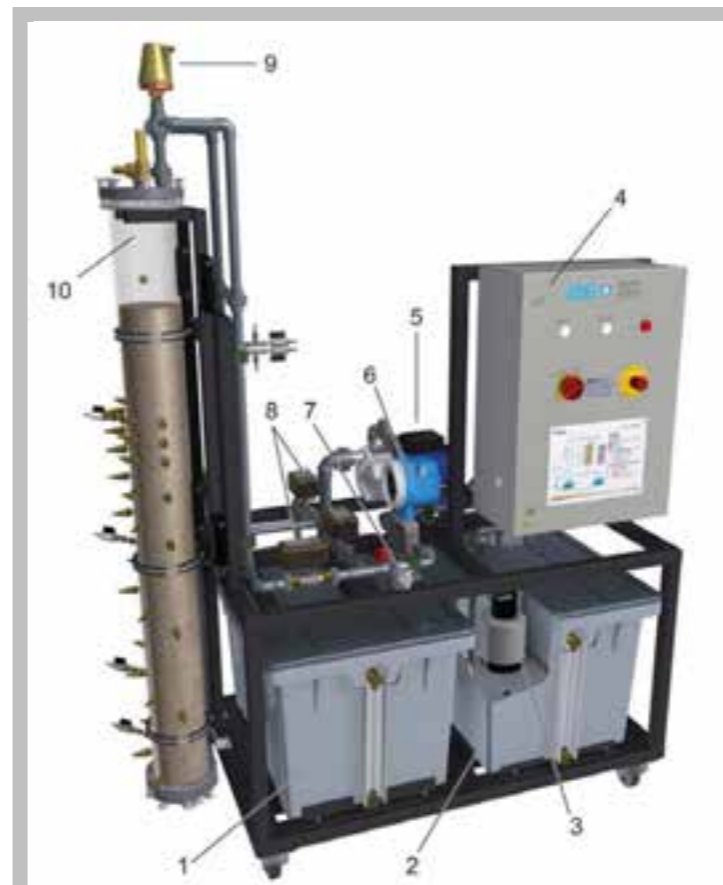
1 treated water tank, 2 raw water tank, 3 raw water pump, 4 switch cabinet, 5 backwash pump, 6 electromagnetic flow rate sensor, 7 temperature sensor, 8 ball valves with electric drive, 9 bleed valve, 10 sand filter
