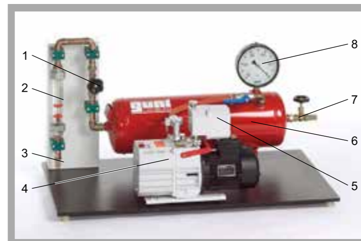
1 needle valve, 2 flow meter, 3 silencer, 4 rotary vane pump, 5 oil separator, 6 pressure vessel, 7 needle valve with silencer, 8 manometer
