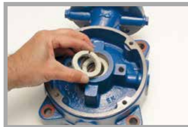
Assembly of the four-stage centrifugal pump: assembling the packing gland rings
