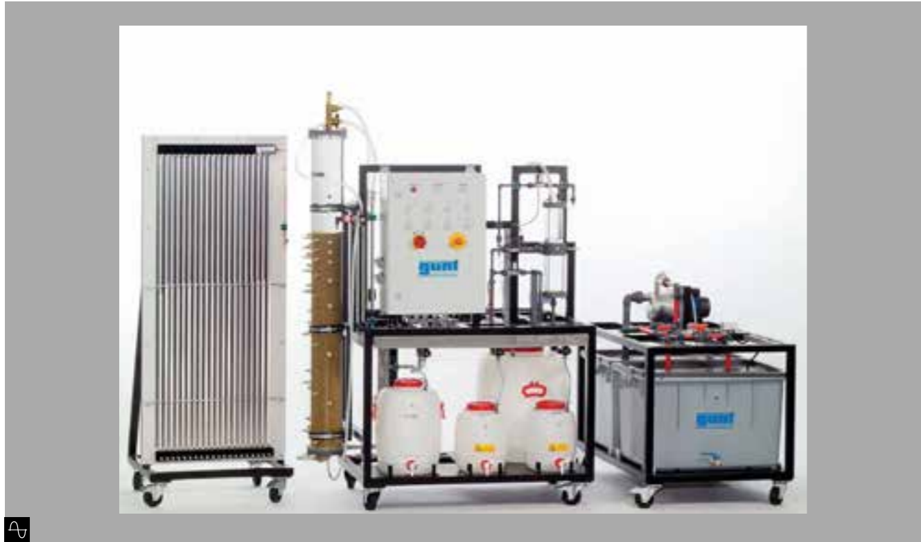
The illustration shows from left to right: manometer panel, trainer, supply unit.
