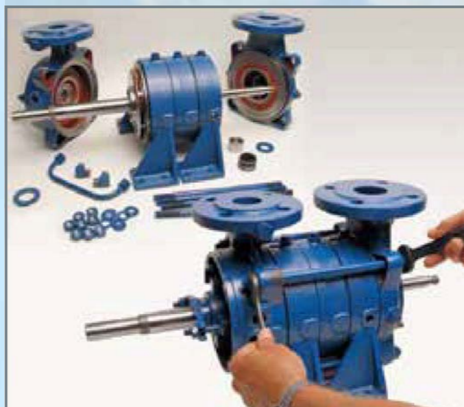
MT 181 Assembly & Maintenance Exercise: Multi-Stage Centrifugal Pump
