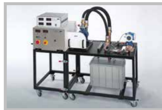
Functional experimental set-up: HM 365 drive unit (left), HM 365.10 with pump to be examined (right)
