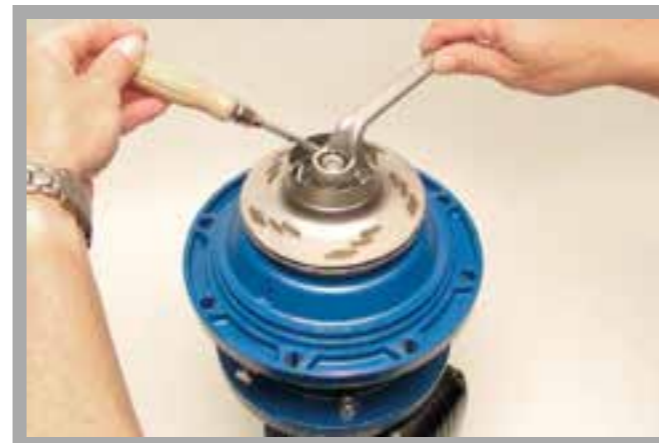
Assembly of the in-line centrifugal pump: tightening the impeller nut
