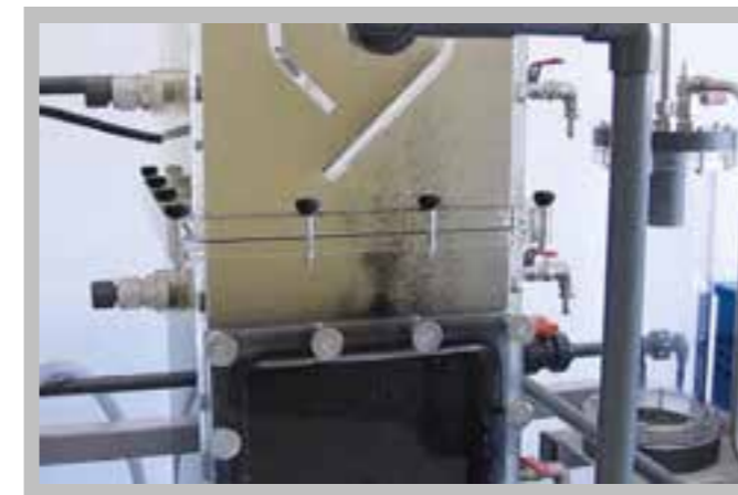
UASB reactor during experimental operation
