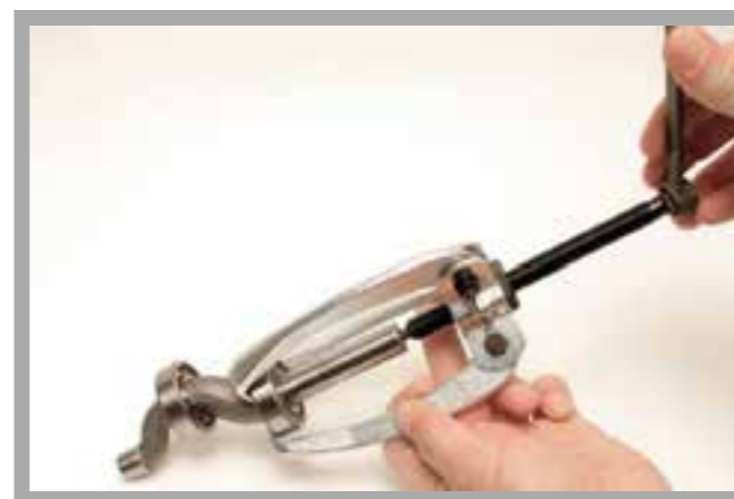
Dissassembly of the piston pump: pulling off the ball bearing of the eccentric shaft (using a bearing puller)
