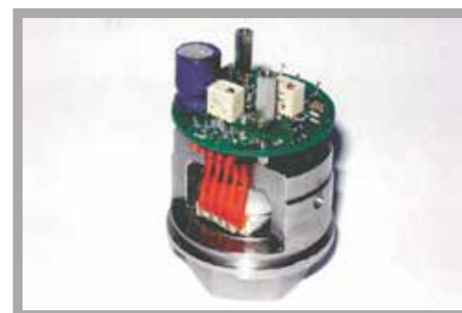
Interior layout of an electronic pressure sensor
