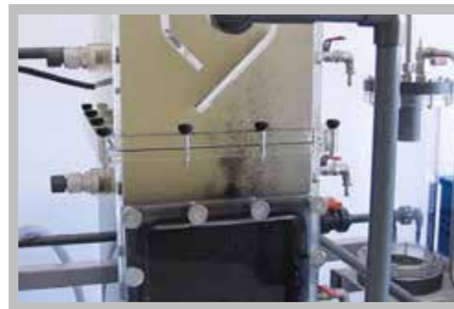
UASB reactor during experimental operation
