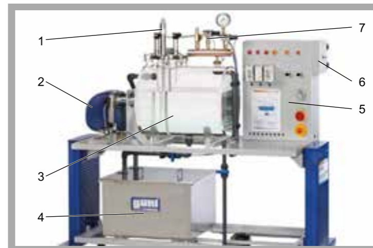
1 water level monitoring, 2 burner, 3 steam boiler model, 4 supply tank, 5 switch cabinet, 6 switch box for fault circuit, 7 pressure measurement equipment
