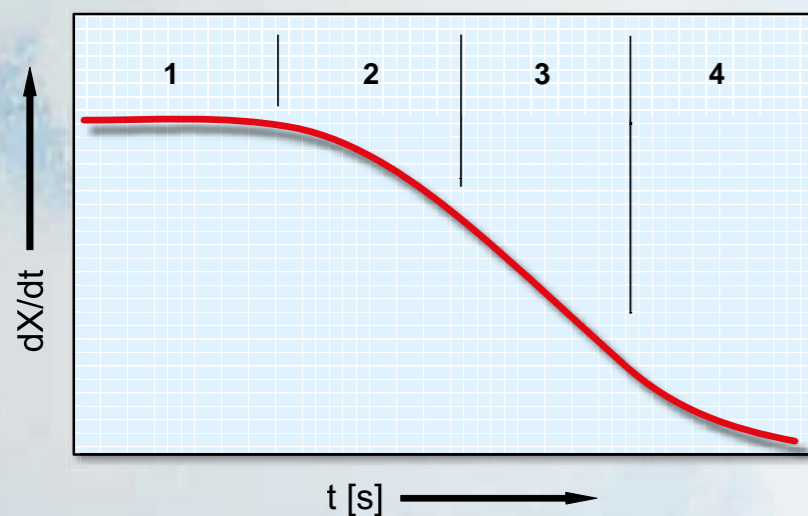
Drying characteristics of a solid with division into drying sections (1-4): dX/dt drying rate, X moisture content [kg (water)/kg (dry solid)], t drying time; 1 surface moisture, 2 capillary moisture, 3 pore moisture, 4 moisture in crystal structure
