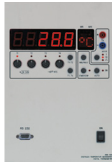
Digital thermometer, CPS
