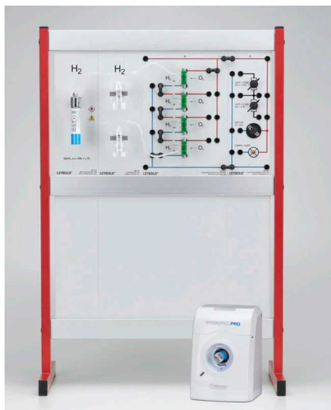
Experiment set-up (C4.4.7.1) for investigations with PEM fuel cells from the Chemistry Experiments catalogue.
