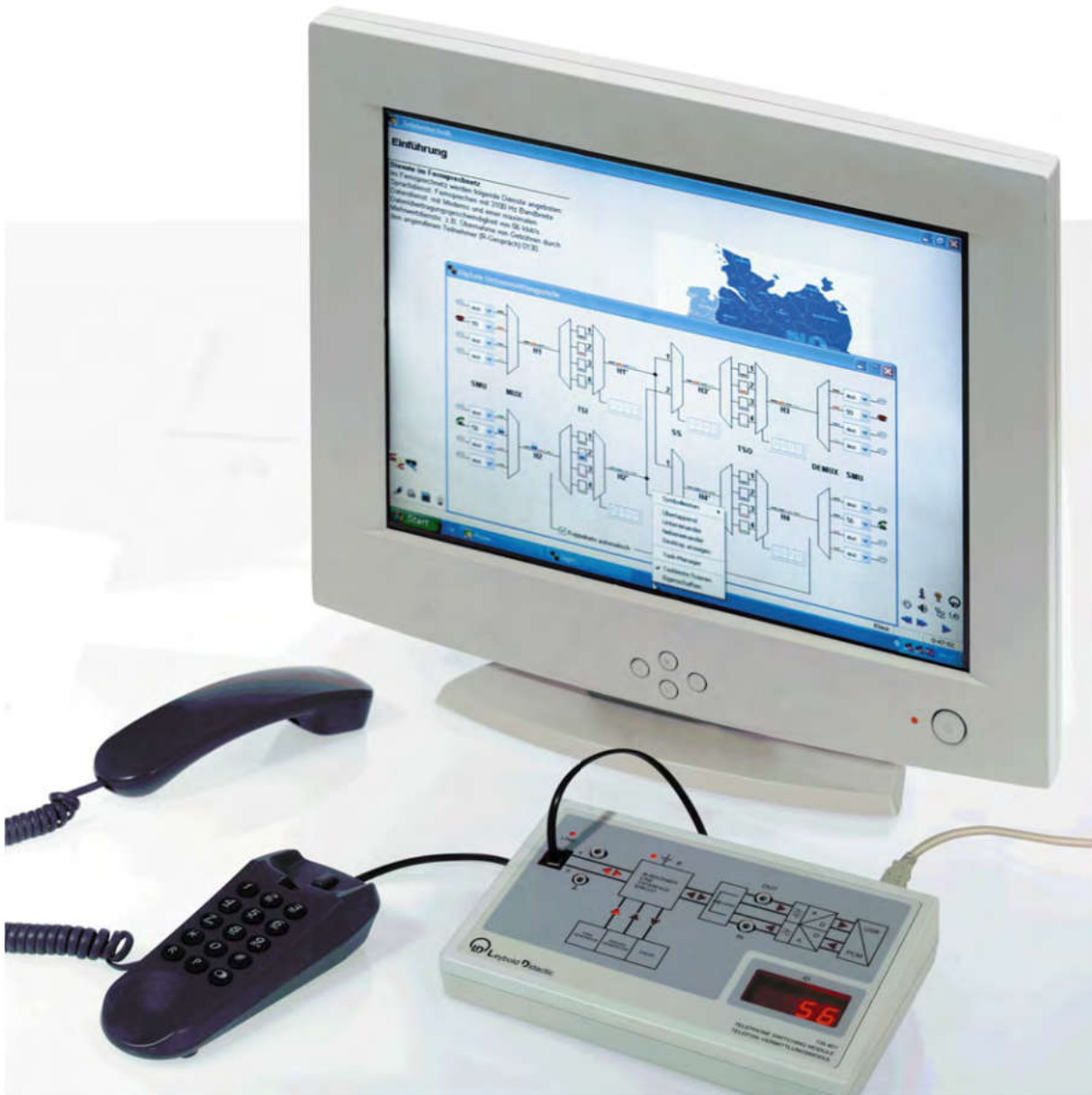
Experiment setup with switching module and telephone
