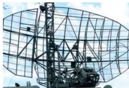
The radar operating frequency defines its range. Long-range radars operate at low frequencies and require large aerials.
