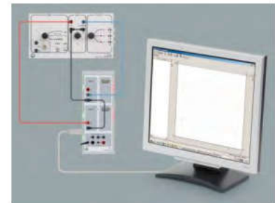
CASSY Lab 2 Plotting the LED characteristics
