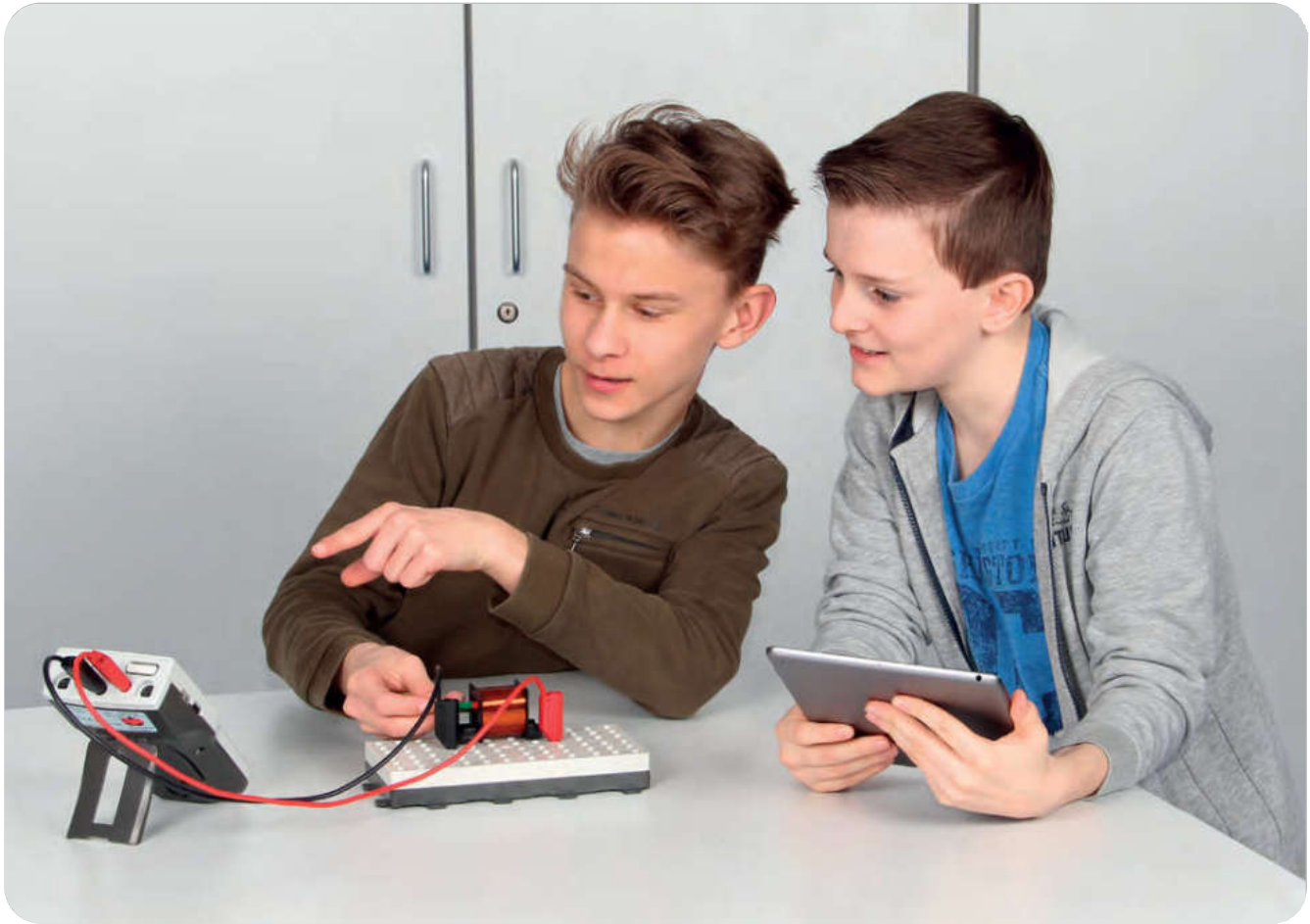
LP3.4.3.1C Electromagnetic induction with bar magnet and a coil
