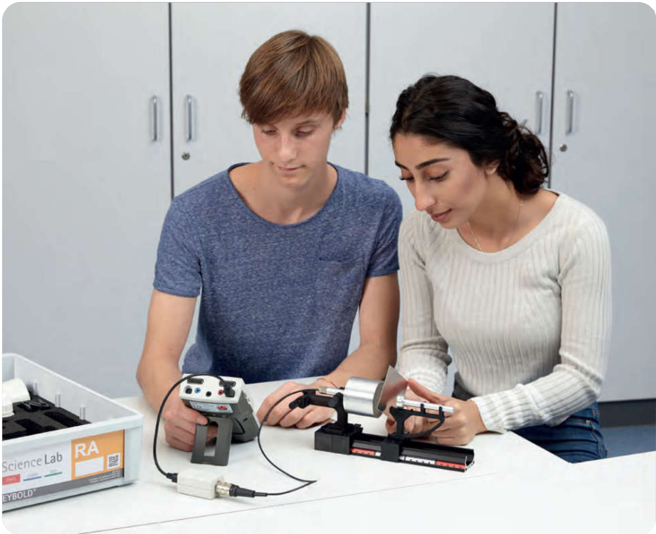
LP6.2.1.3C Detecting radioactive radiation in a button shaped source
