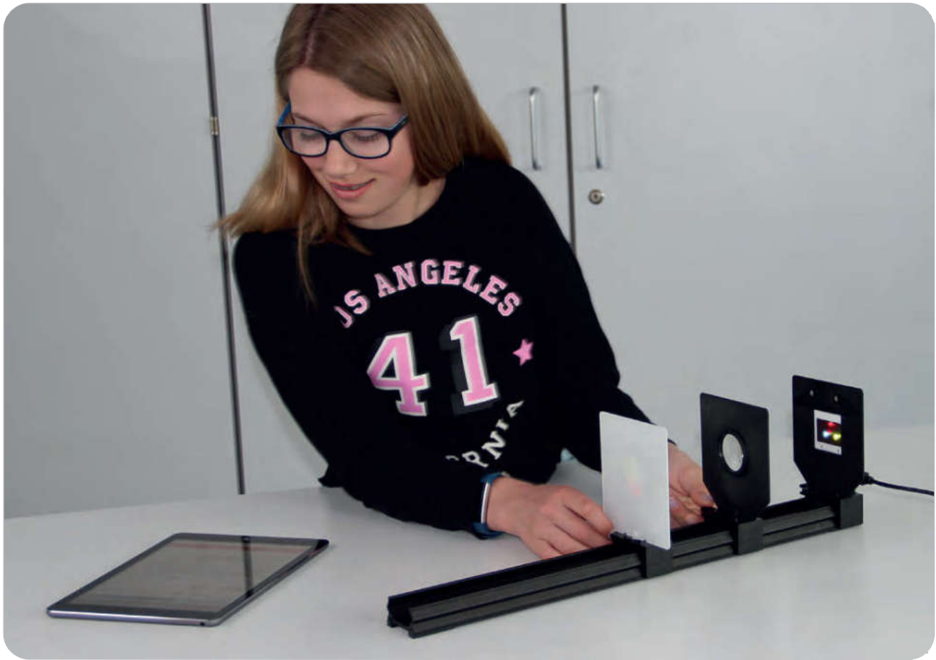
LP5.2.3.4 Additive mixing of three light colours
