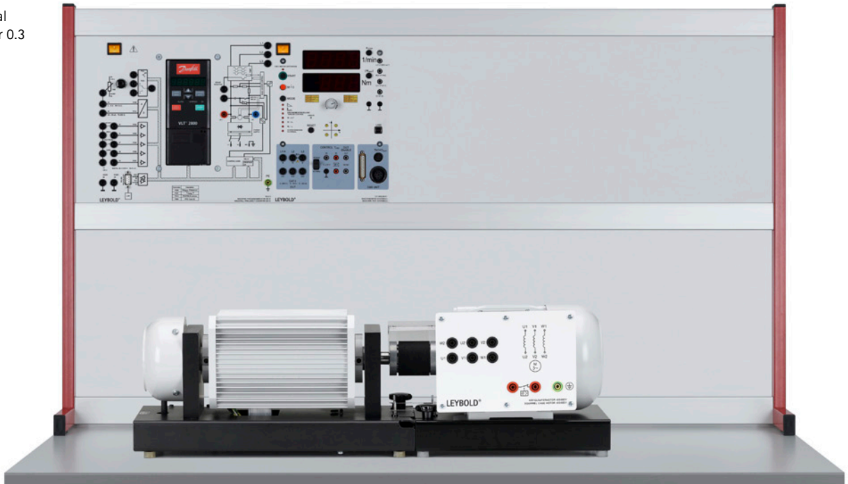
Drives with Industrial Frequency Converter 0.3 (E2.5.3.4)
