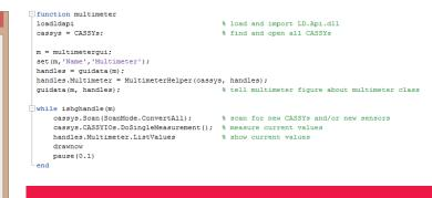
The ready-to-use multimeter example supports all CASSYs and most sensors and sensor boxes, including all measurement parameters and measurement ranges.
