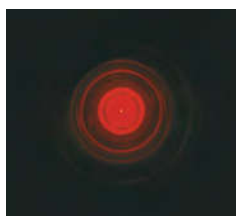
Optical analog of Debye-Scherrer diffraction (P6.1.5.2)
