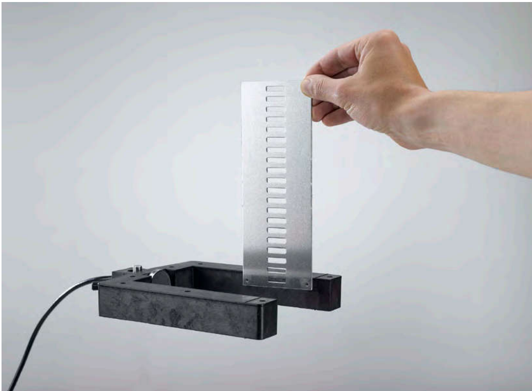
Free fall: multiple measurements with the g ladder (P1.3.5.3)
