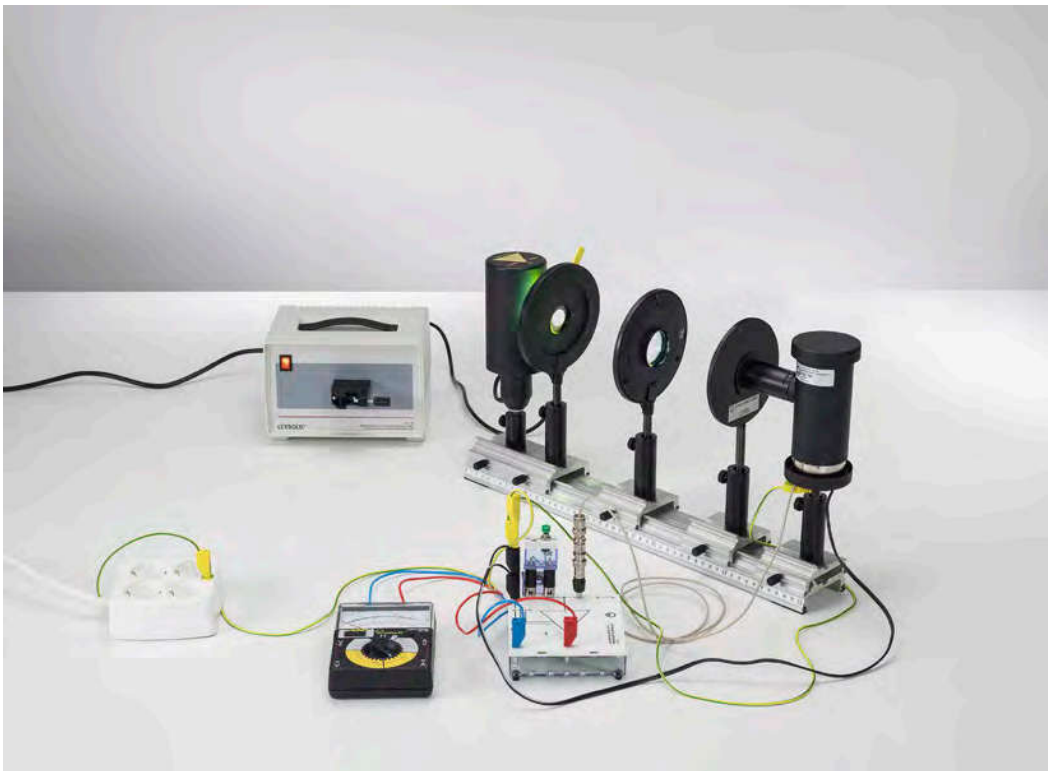
Determining Planck's constant - Selection of wavelengths using interference filters on the optical bench (P6.1.4.3)
