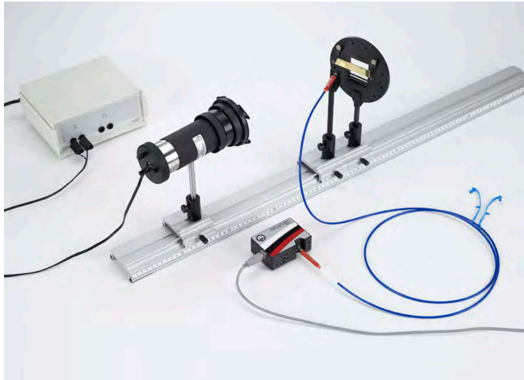
Reflection spectra of different materials - Recording and evaluating with a spectrophotometer (P5.2.5.1)
