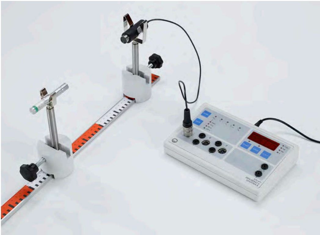
Confirming the inverse-square law of distance for \beta radiation (P6.4.4.3)
