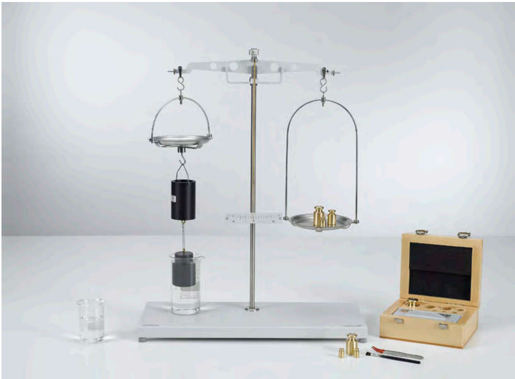
Confirming Archimedes' principle (P1.8.2.1)
