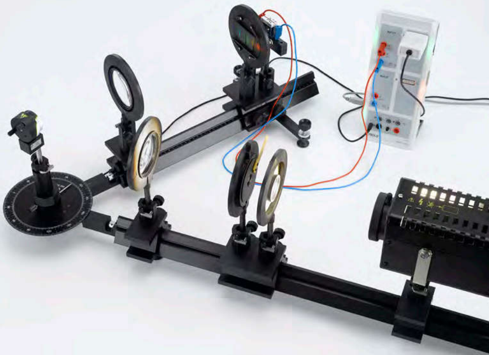
Investigating the spectrum of a xenon lamp with a holographic grating (P5.7.2.5)
