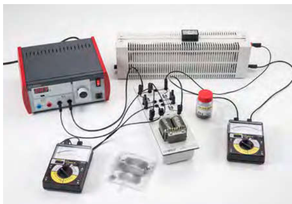
Voltage transformation with a transformer under load (P3.4.5.2)
