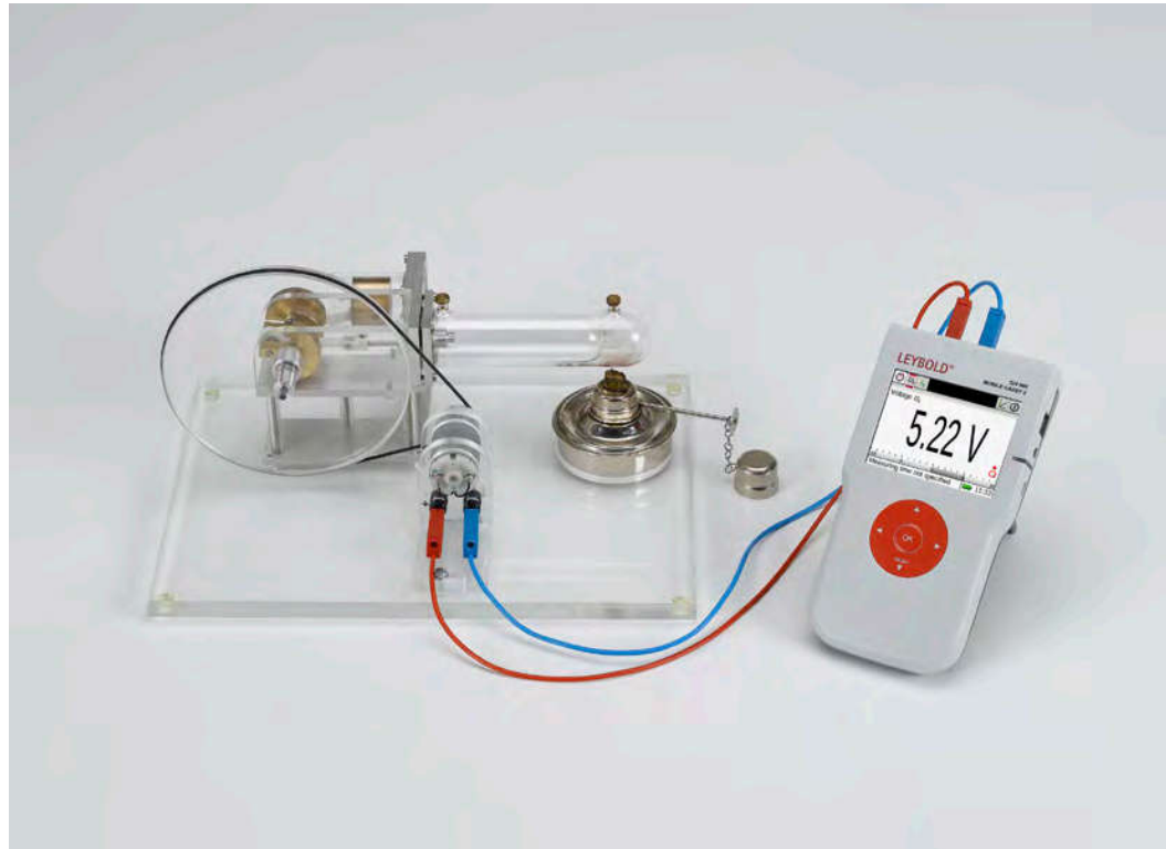
Operating the hot-air engine P as a thermal engine (P2.6.1.5)
