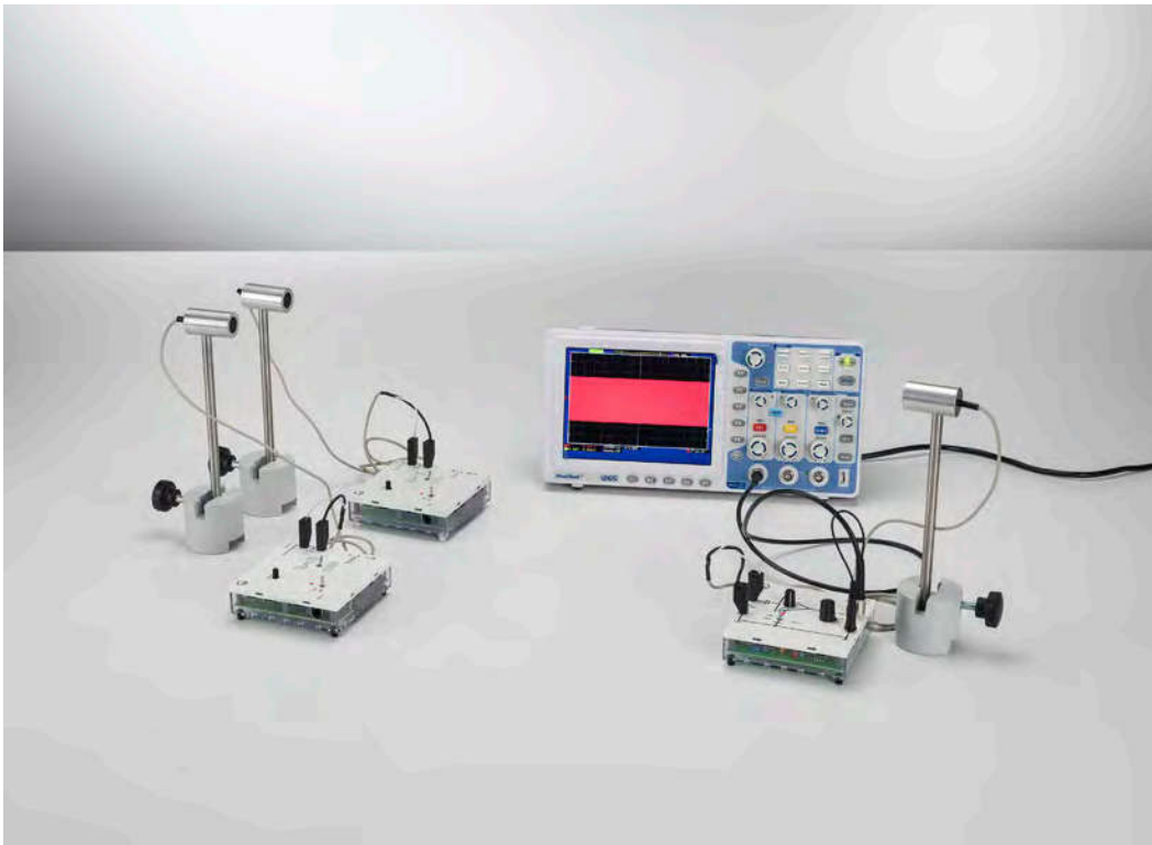
Beating of ultrasonic waves (P1.7.5.1)
