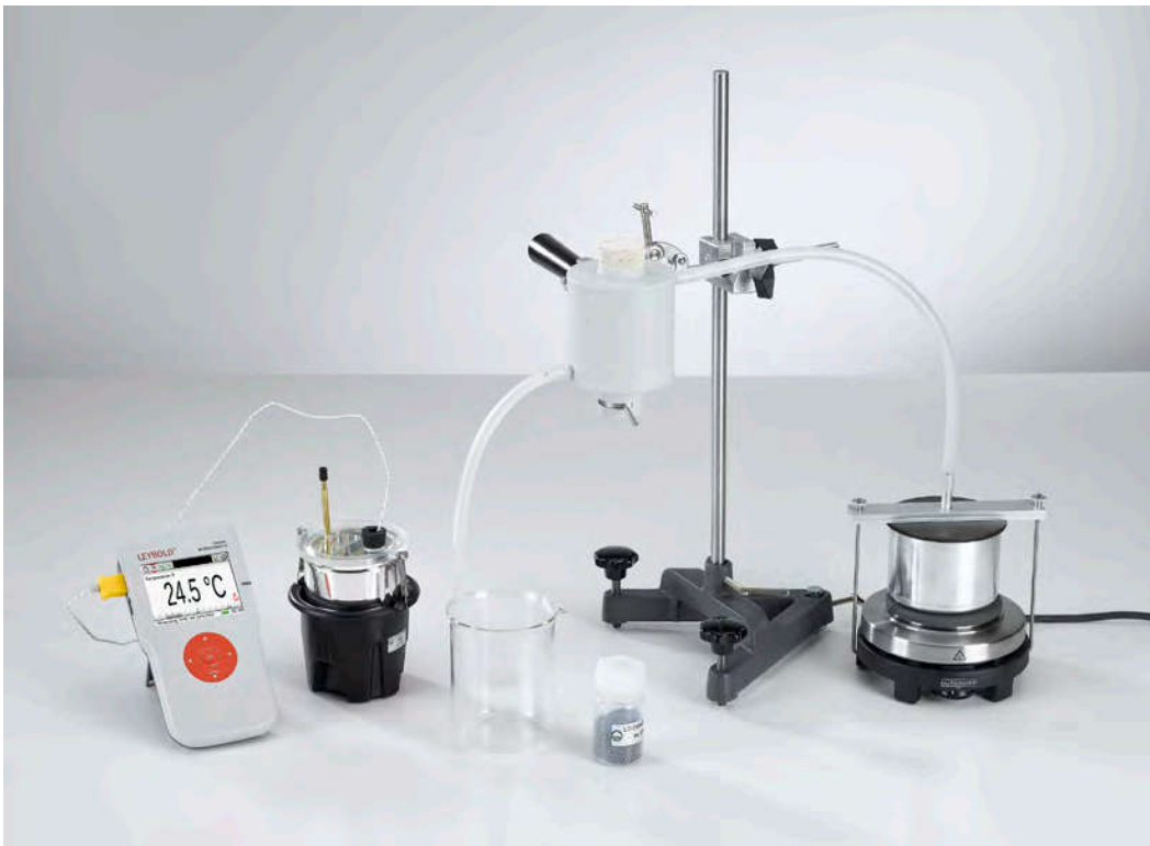
Determination of specific heat of solids - Measuring with Mobile-CASSY (P2.3.2.2)
