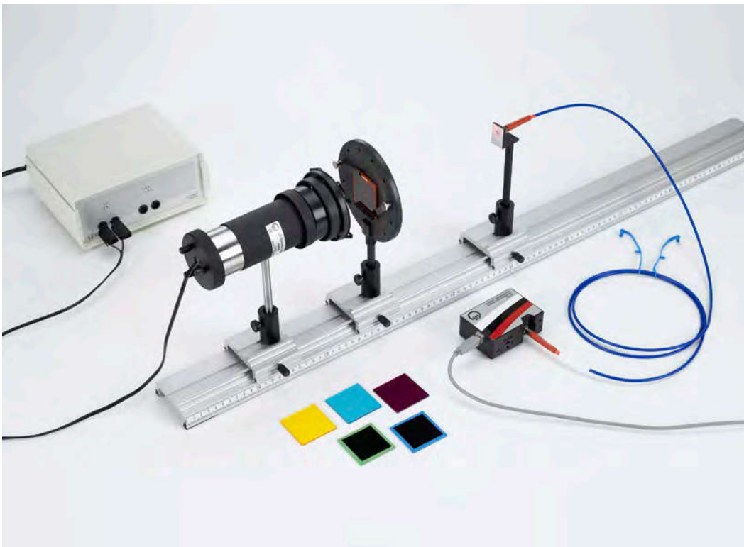
Absorption spectra of tinted glass samples - Recording and evaluating with a spectrophotometer (P5.2.4.3)
