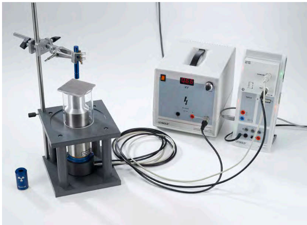
Absorption of \gamma radiation (P6.5.5.3)
