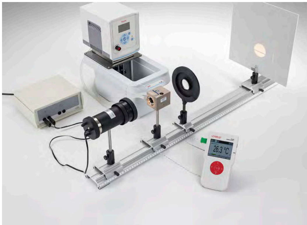
Observing a mixture of liquid and gas at the critical point - Measuring with Mobile-CASSY (P2.4.3.2)
