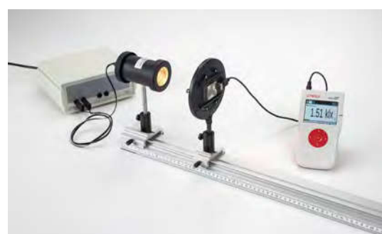
Determining the luminous intensity as a function of the distance from the light source - Measuring with Mobile-CASSY (P5.5.1.2)
