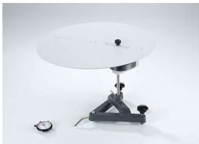
Confirming Steiner's theorem (P1.4.5.3)
