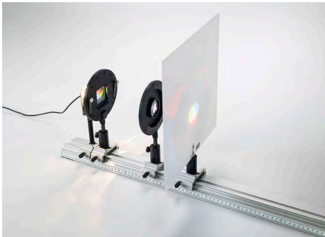
Demonstration of additive color mixing (P5.2.3.2)
