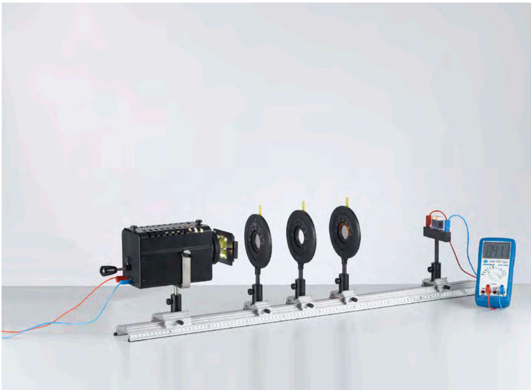
Quarter-wavelength and half-wavelength plate (P5.4.2.2)
