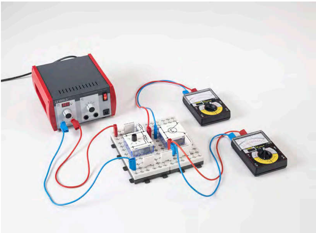
Recording the characteristics of a transistor (P4.1.5.2)
