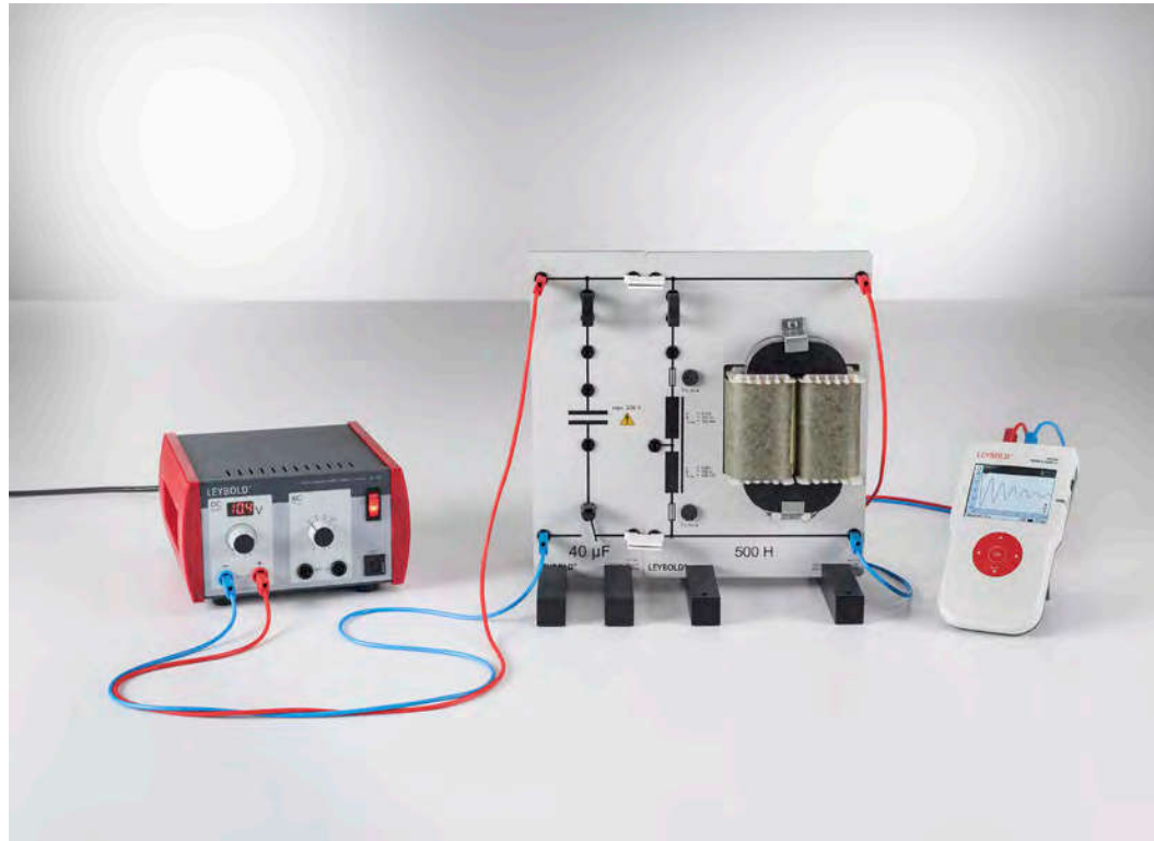
Free electromagnetic oscillations (P3.7.1.1)
