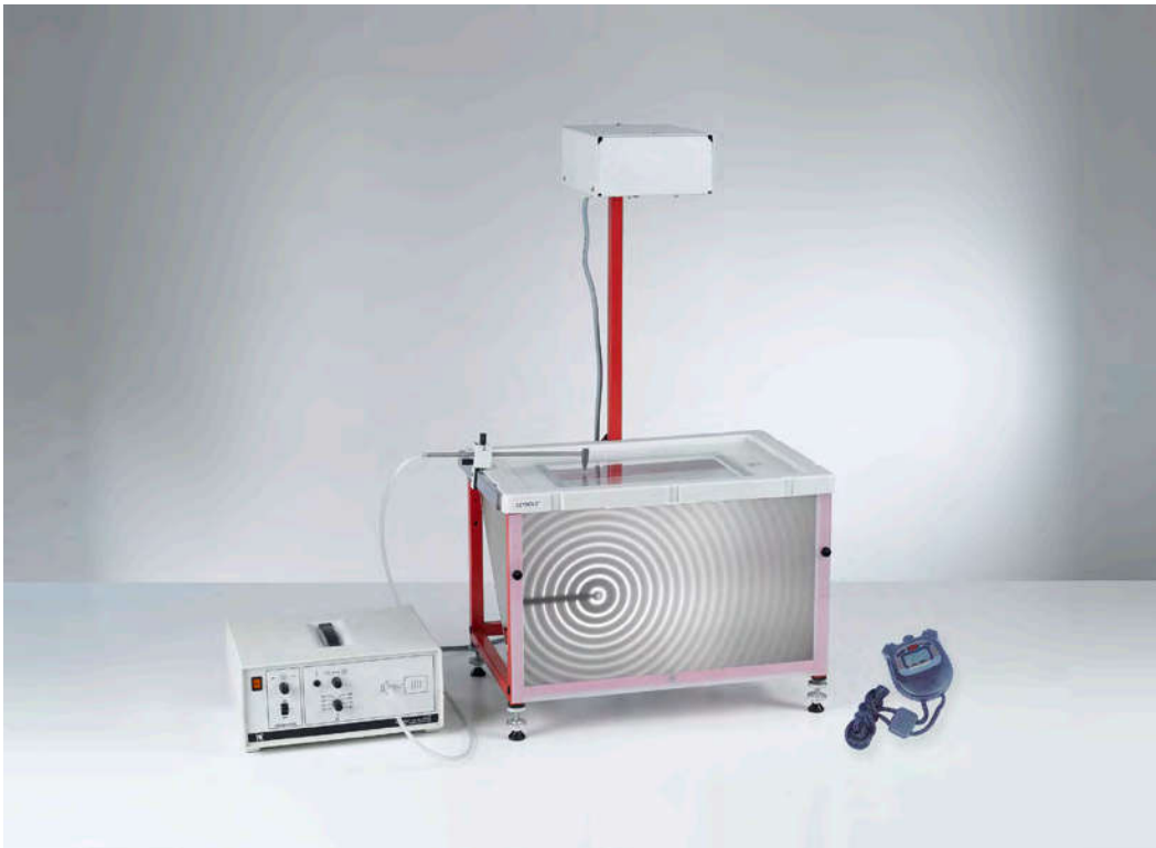
Exciting circular and straight water waves (P1.6.4.1)
