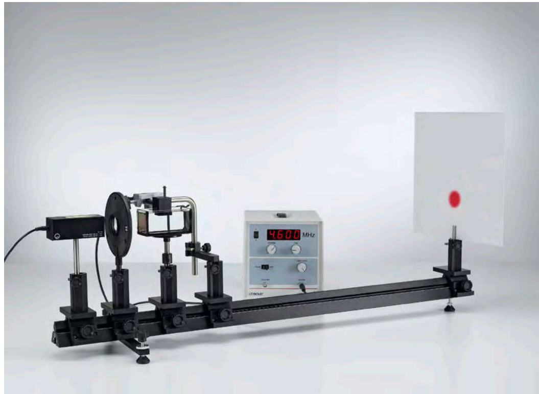
Determination of the velocity of sound in liquids - standing ultrasonic waves as optical grating (P1.7.8.1)
