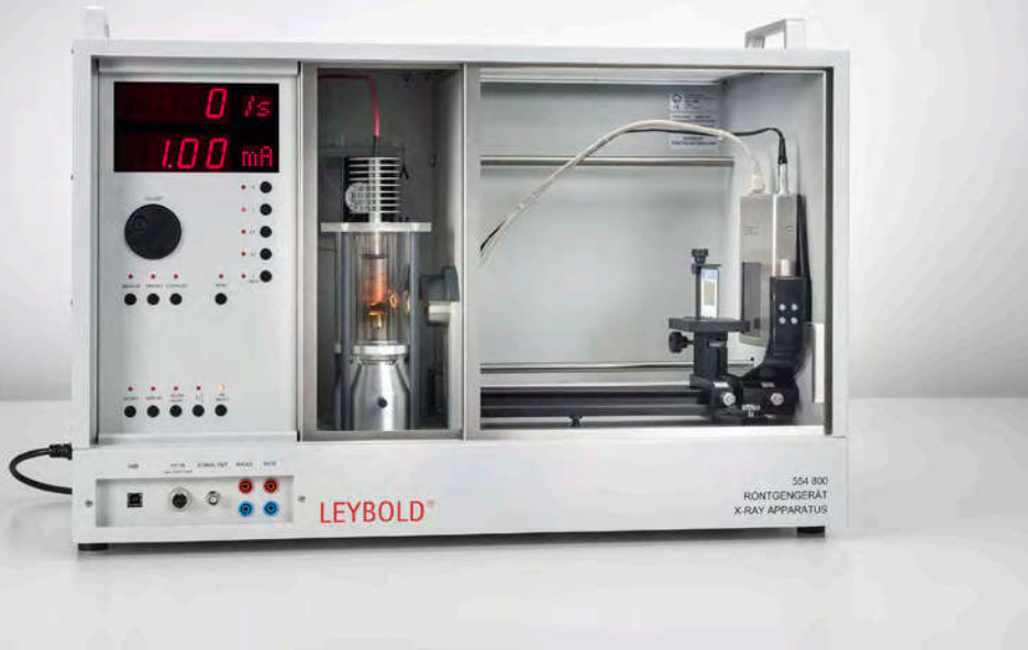
Digital X-ray photography with the X-ray image sensor (P6.3.1.12)
