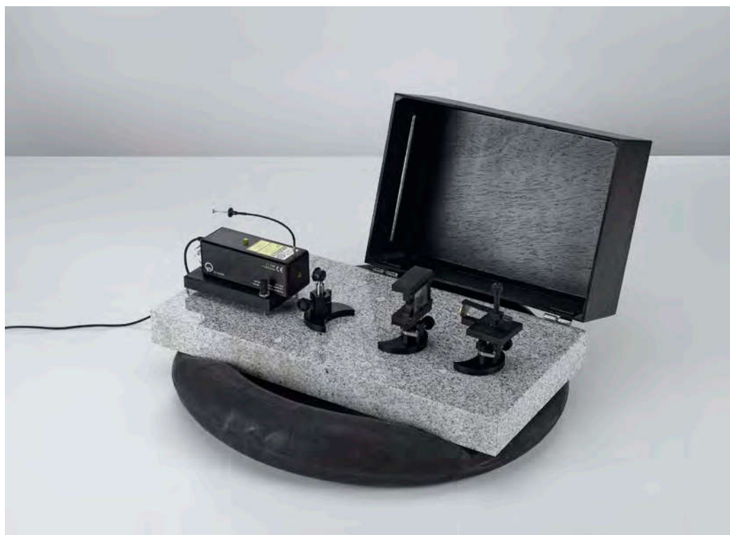
Creating white-light reflection holograms on the laser optics base plate (P5.3.6.1)
