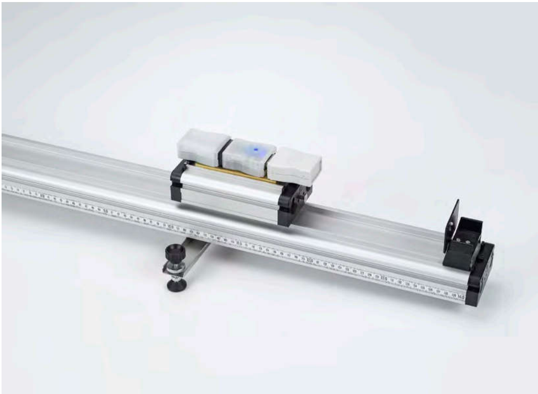
Accelerated motions with an acceleration sensor (P1.3.2.5)
