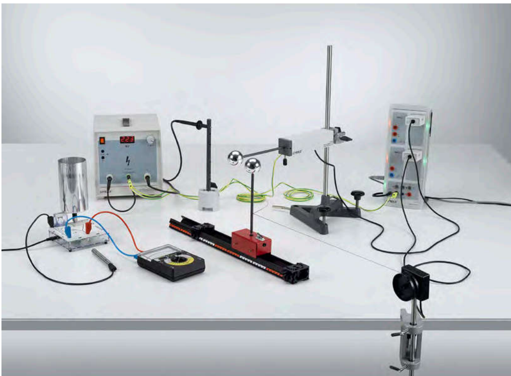
Confirming Coulomb's law - Recording and evaluating with CASSY (P3.1.2.3)
