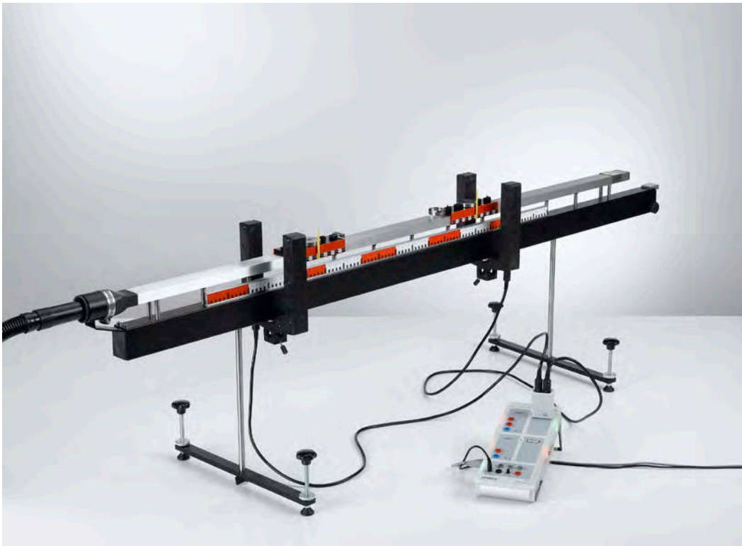
Energy and linear momentum in elastic and inelastic collision on the linear air track - Measuring with two forked light barriers and CASSY (P1.3.4.8)
