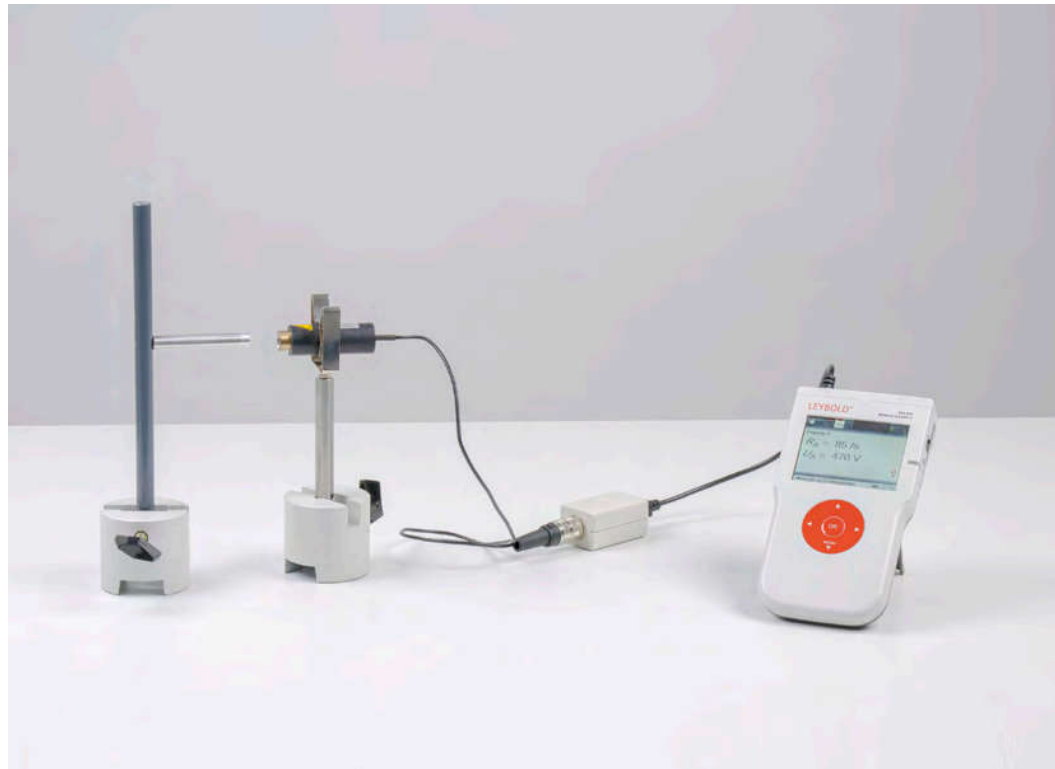
Recording the characteristic of a Geiger-Müller (end-window) counter tube (P6.4.1.4)
