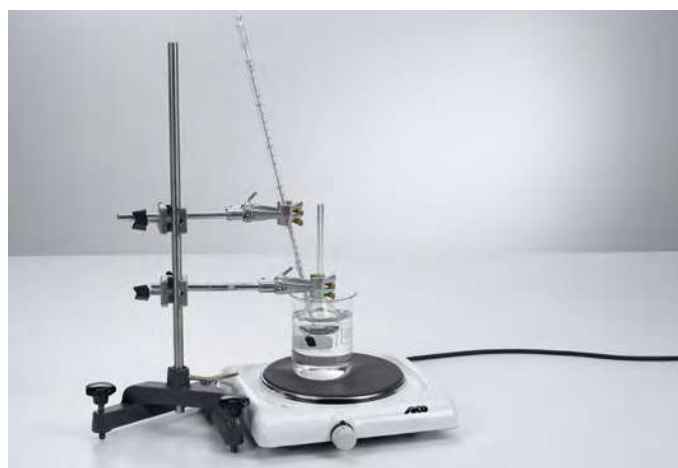
Determination of volumetric expansion coefficient of liquids (P2.1.2.1)
