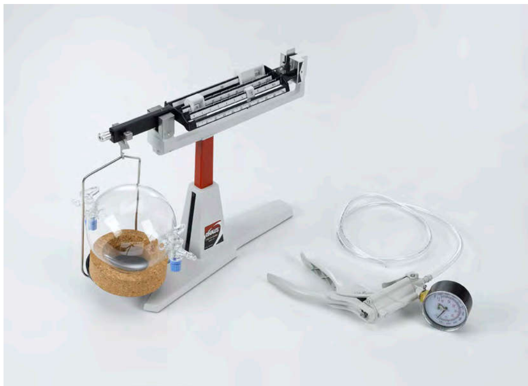
Determining the density of air (P1.1.2.4)
