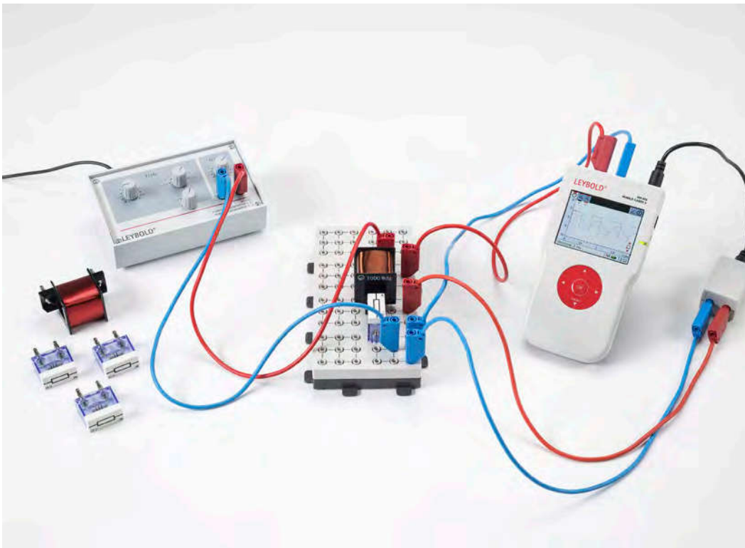
Measuring the current in a coil when switching DC on and off - Measuring with Mobile-CASSY (P3.6.2.3)
