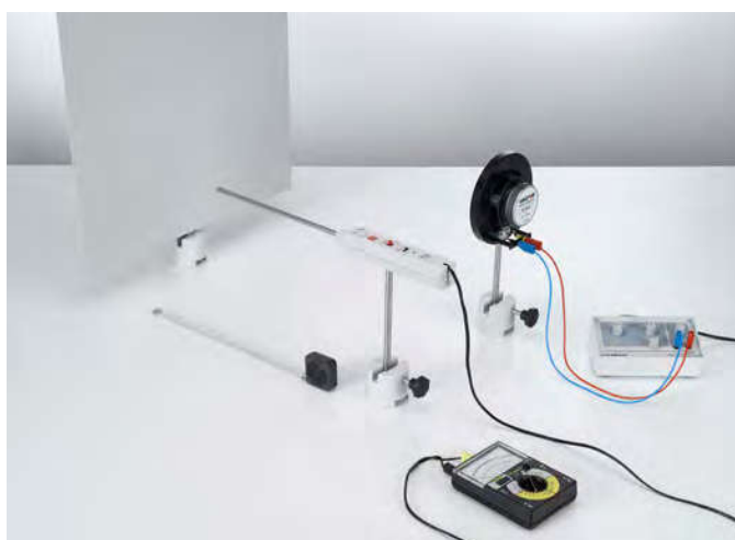
Determining the wavelength of standing sound waves (P1.7.3.2)
