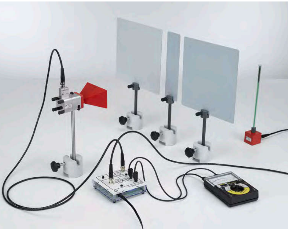
Diffraction of microwaves (P3.7.4.4)
