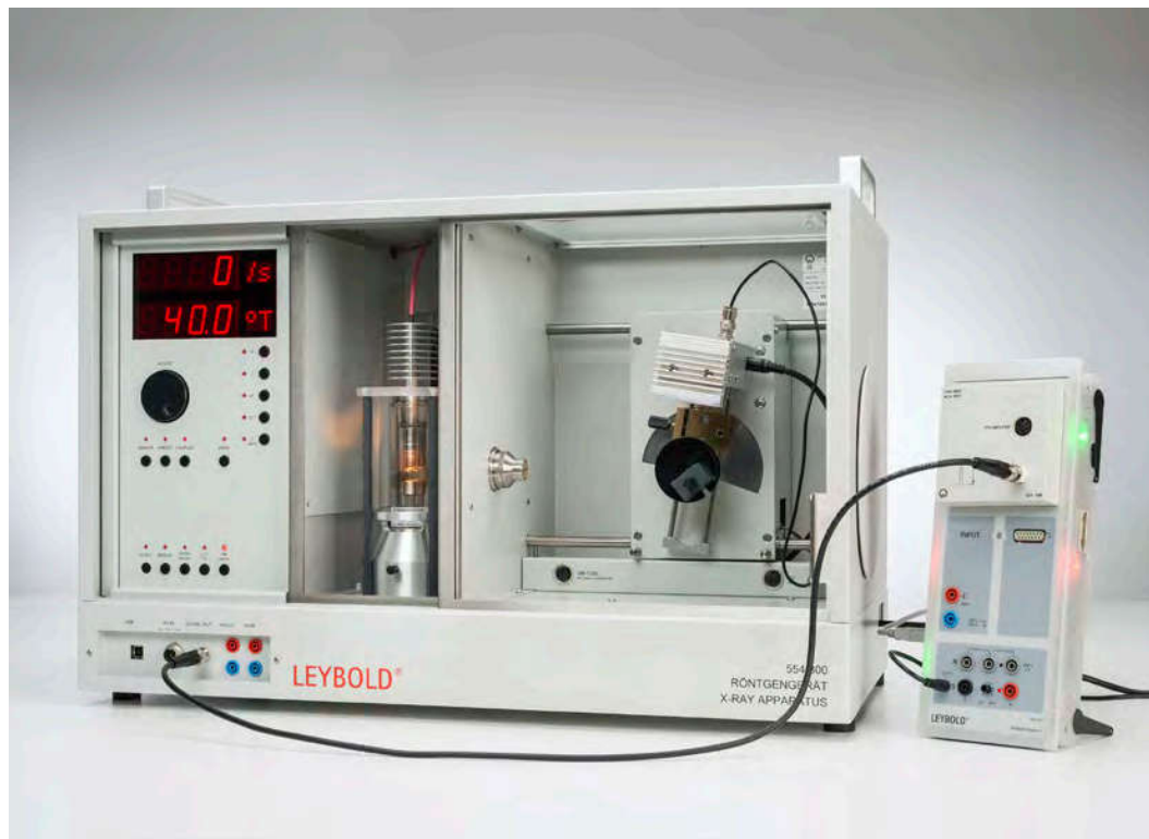
Recording and calibrating an X-ray energy spectrum (P6.3.5.1)
