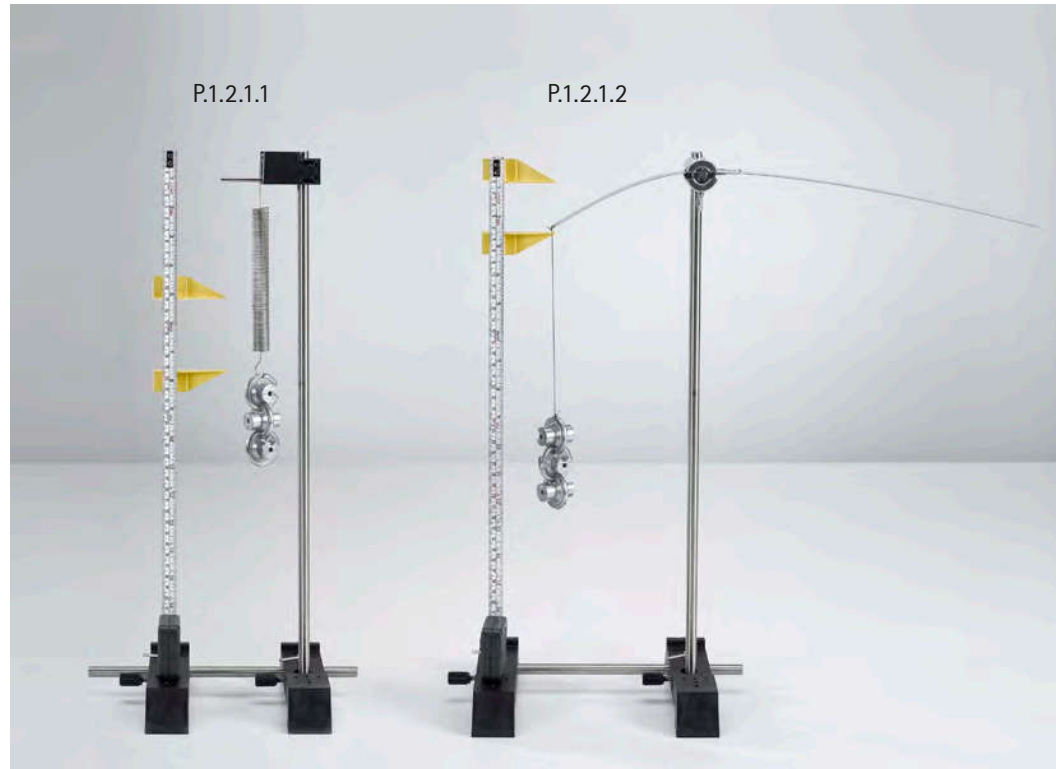
Expansion of a helical spring (P1.2.1.1)
