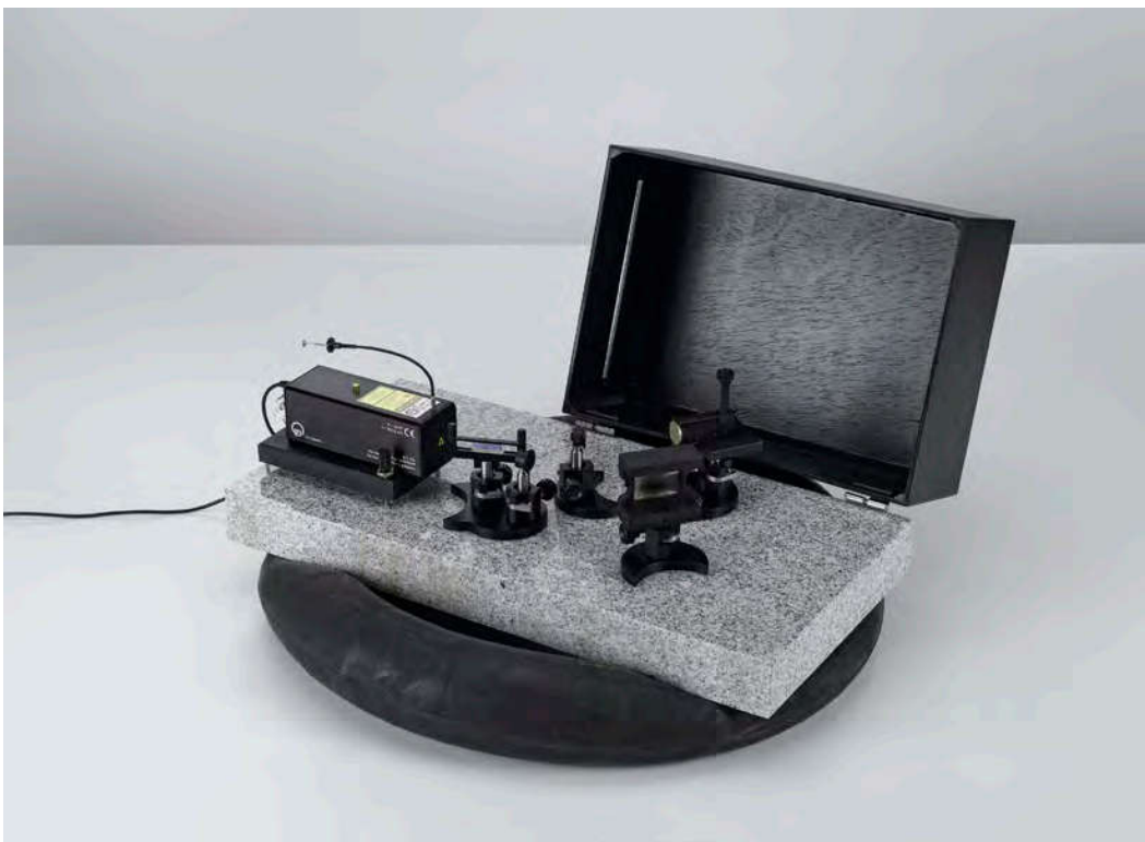
Creating transmission holograms on the laser optics base plate (P5.3.7.1)
