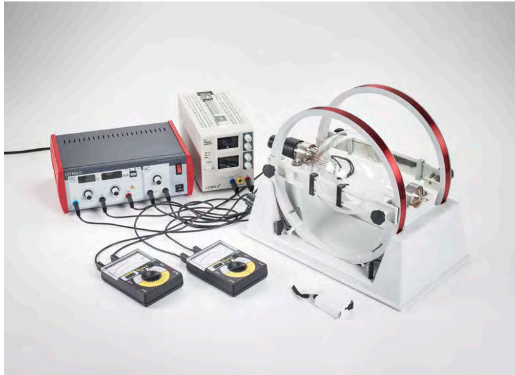
Determining the specific charge of the electron (P6.1.3.1)
