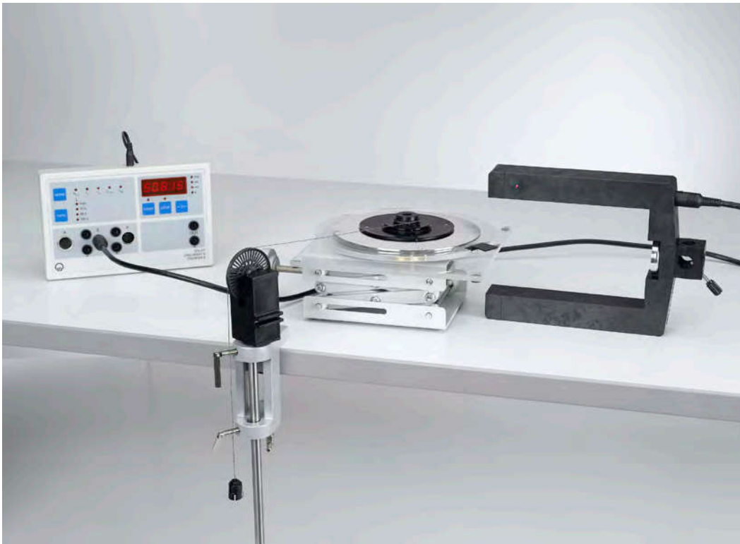
Path-time diagrams of rotational motions - Time measurement with the counter (P1.4.1.1)
