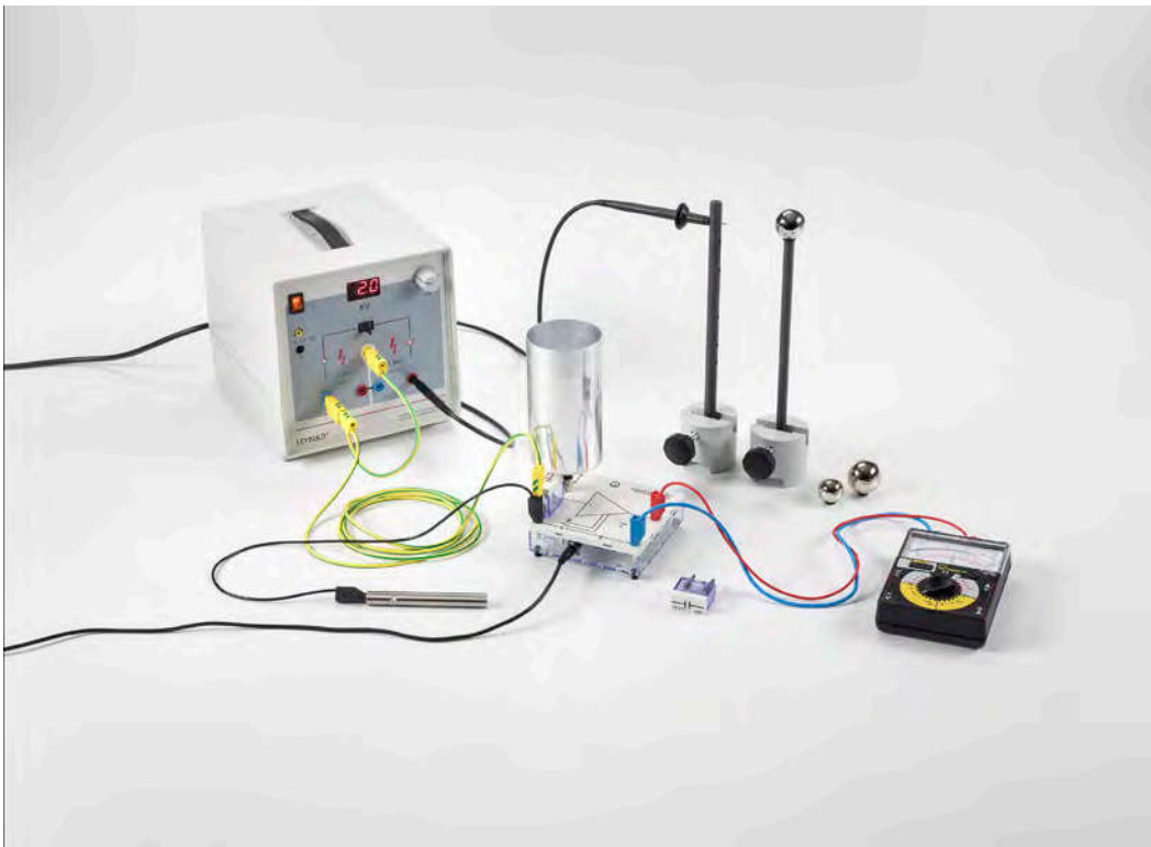
Determining the capacitance of a sphere in free space (P3.1.6.1)
