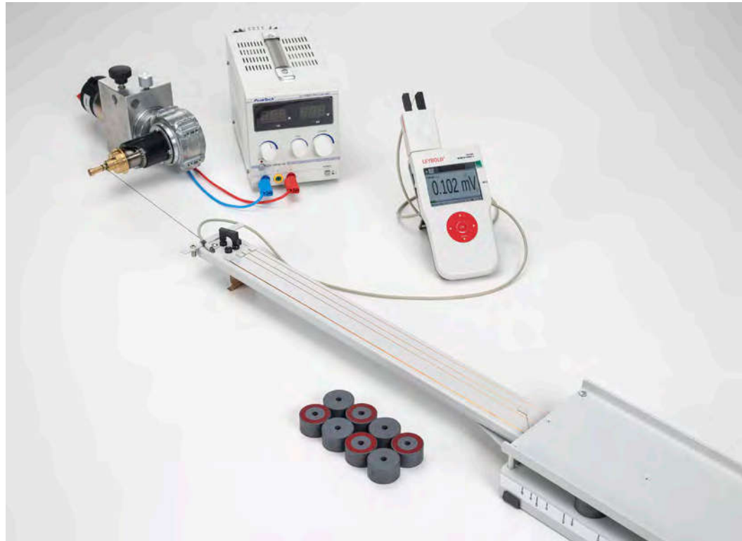
Measuring the induction voltage in a conductor loop moved through a magnetic field (P3.4.2.1)
