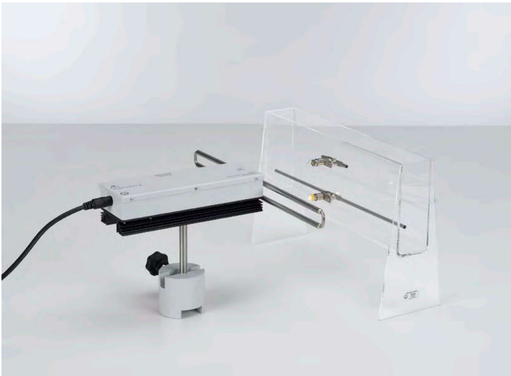
Estimating the dielectric constant of water in the decimeter-wave range (P3.7.2.4)
