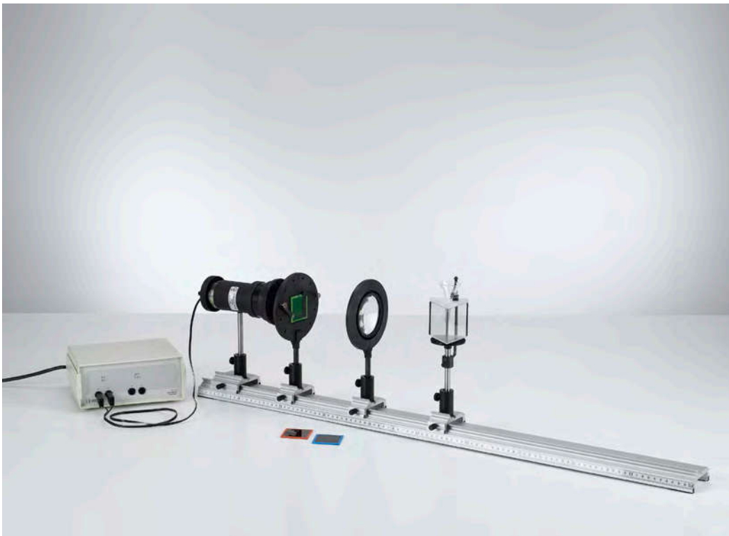
Determining the refractive index and dispersion of liquids (P5.2.1.2)
