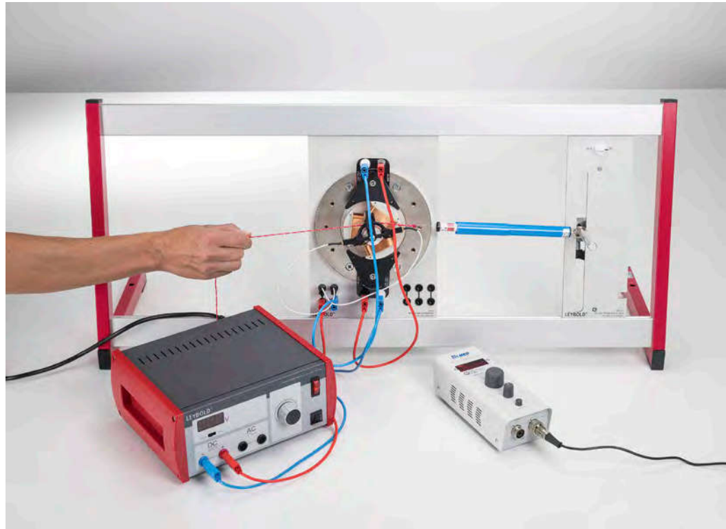
Experiments with a universal motor in shunt connection (P3.5.3.3)
