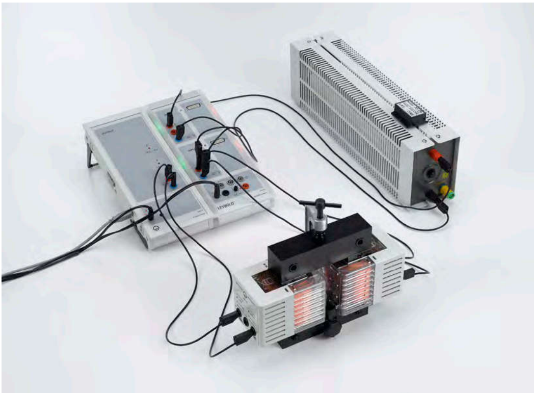
Power transmission of a transformer (P3.4.5.4)
