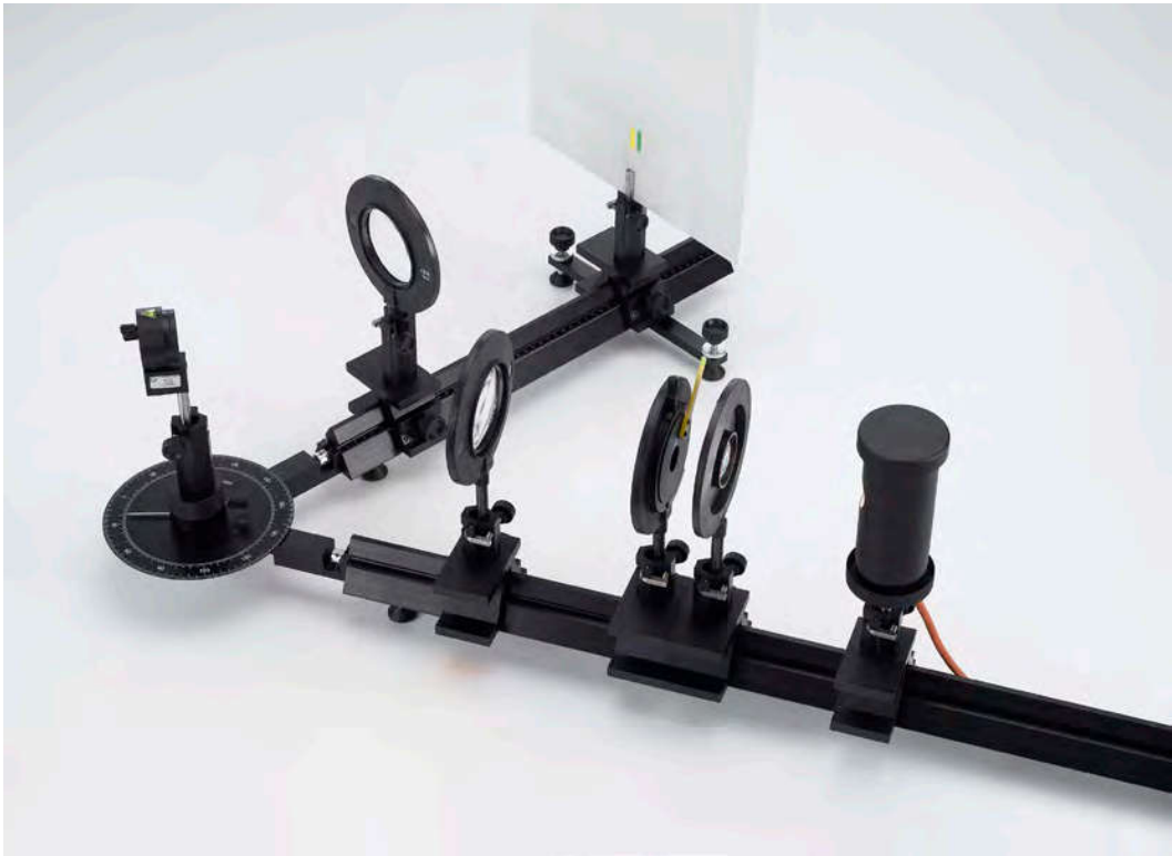
Investigating the spectrum of a high pressure mercury lamp (P6.2.2.3)
