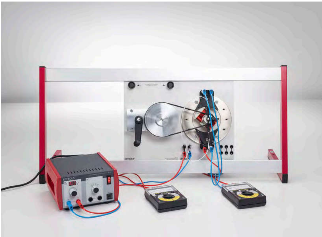
Generating AC voltage using a generator with electromagnetic rotating pole (power-plant generator) (P3.5.2.3)
