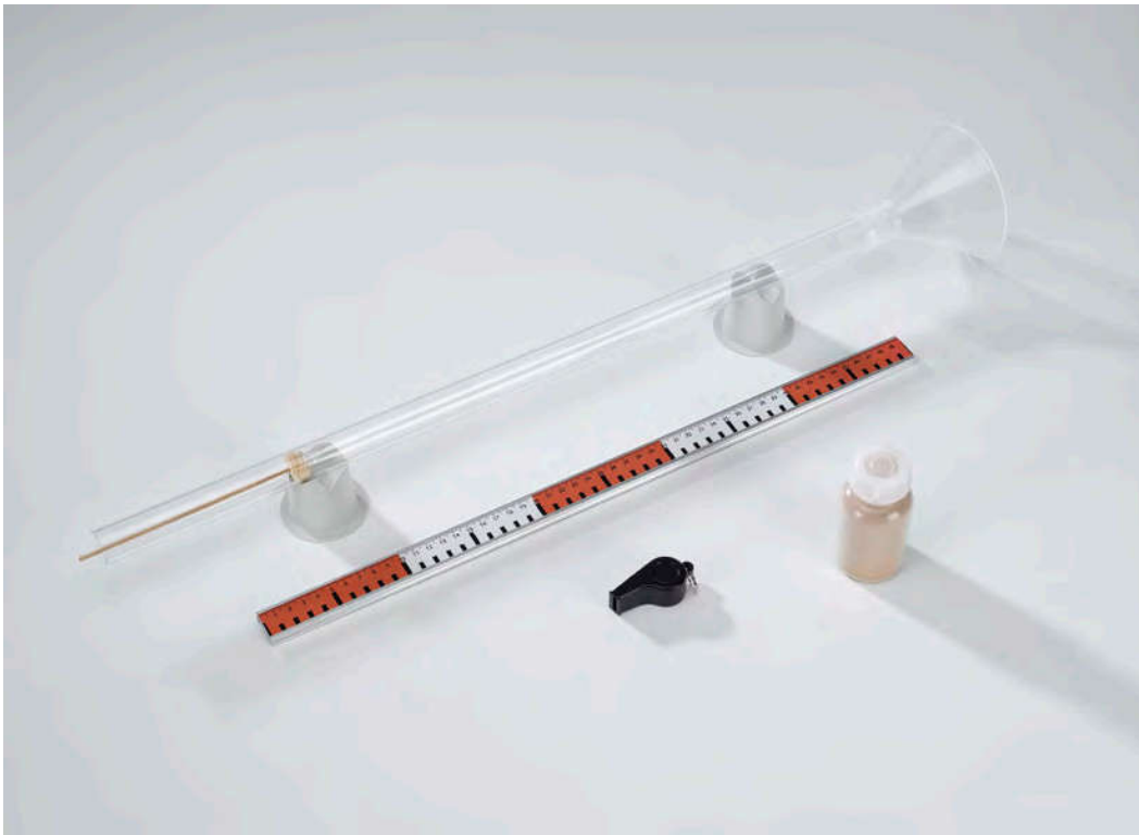
Kundt's tube: determining the wavelength of sound with the cork-powder method (P1.7.3.1)
