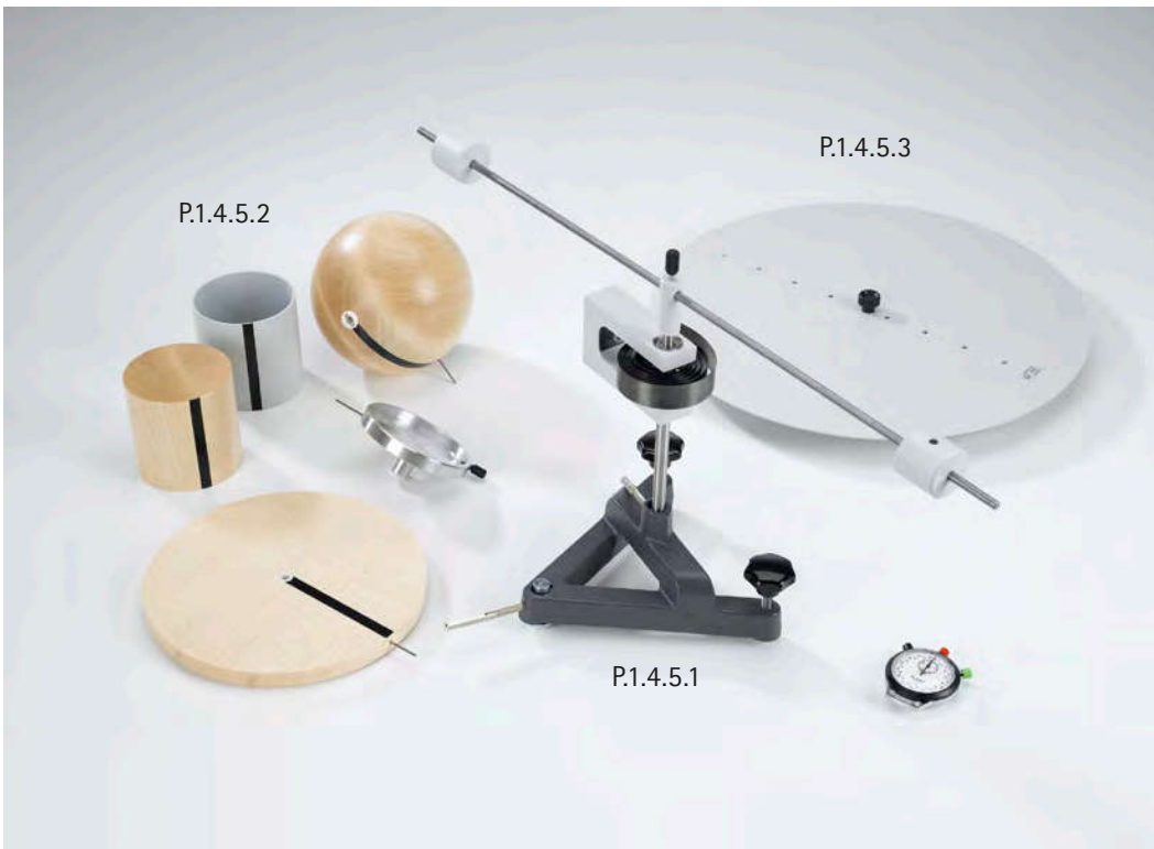
Definition of moment of inertia (P1.4.5.1)
