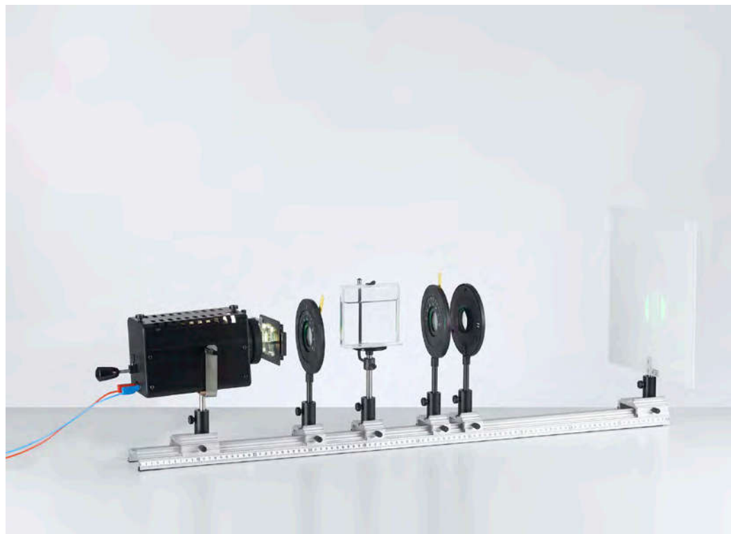
Rotation of the plane of polarization with sugar solutions (P5.4.3.2)
