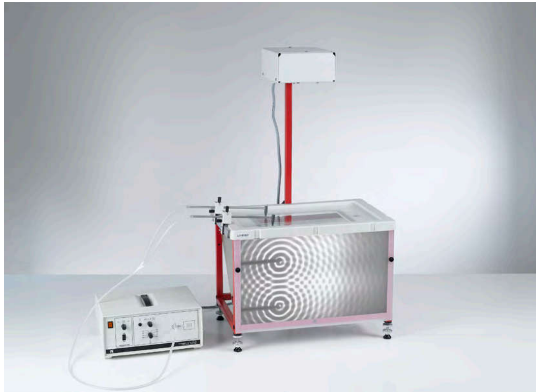
Two-beam interference of water waves (P1.6.5.1)
