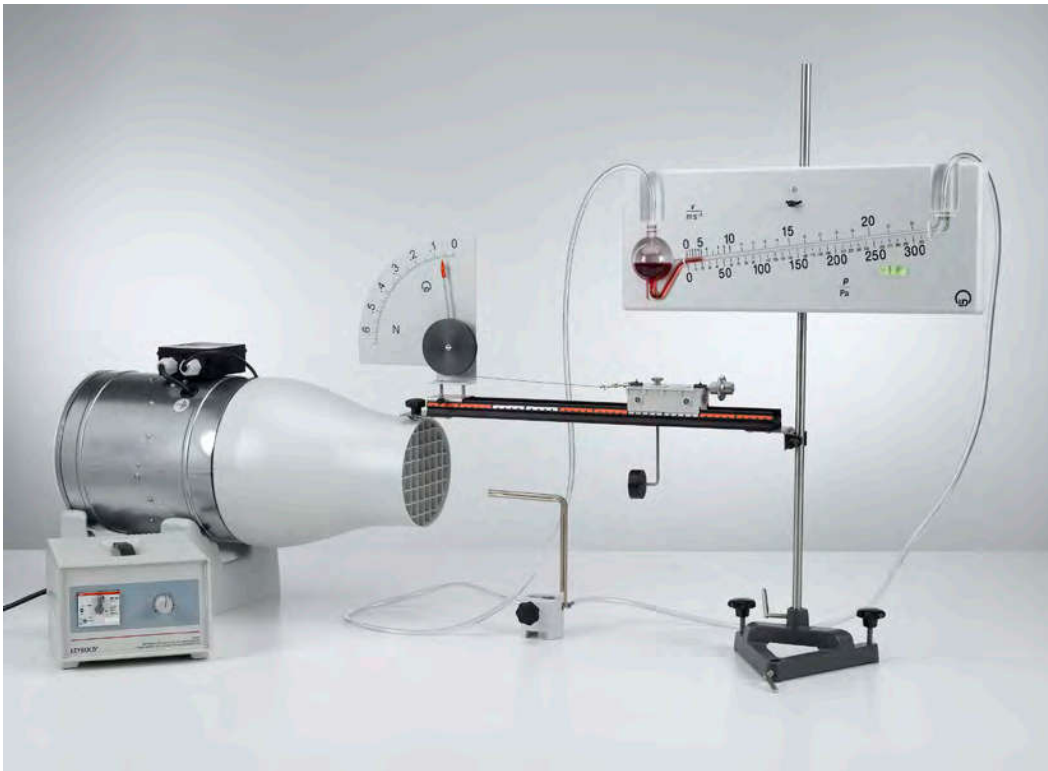
Air resistance as a function of the wind speed and body shape - Measuring the wind speed with the precision manometer (P1.8.6.1)
