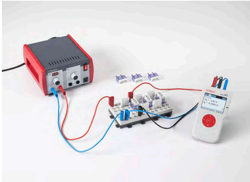
Measuring current and voltage at resistors connected in parallel (P3.2.3.1)
