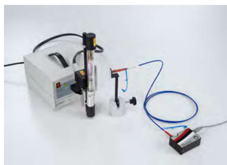
Emission spectrum of atomic hydrogen (P6.2.1.4)
