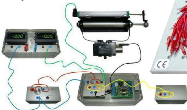
Asservissement de position.
