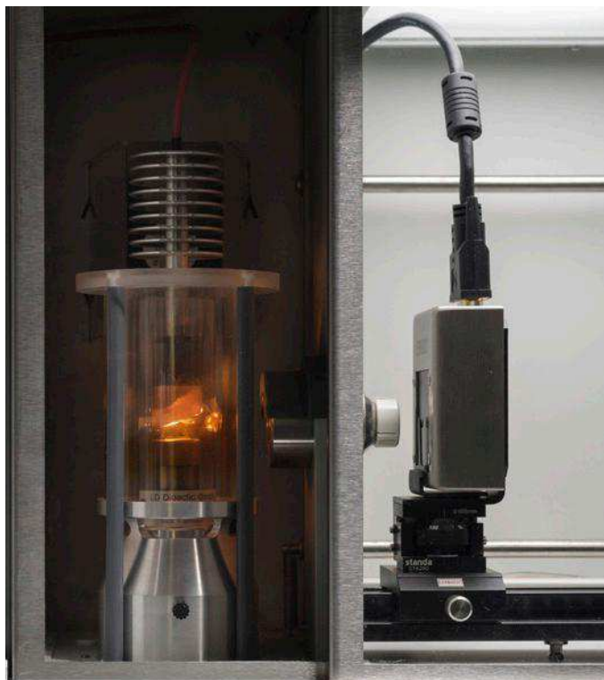
Fast creation of a Laue diagram with the X-ray image sensor.
