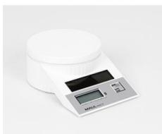
For demonstration and student experiments, with 4-digit LCD display (easy, mirror-free reading through sharply slanted display), automatic switch-off, automatic reset and hold key to freeze the displayed weight. Powered by solar cells, excess energy is stored and used in low light conditions (below 150 lux). Stable housing made of unbreakable plastic. Made in Germany with patented measuring system.
