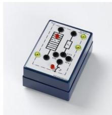
BS 0.4 Current-using equipment with body-contact resistors In addition to the resistance of the current-consuming equipment, 2200 Ohm 25 W, this module includes the following body-contact resistance values selectable by positioning a connecting plug: 470 Ohm, 100 W / 2.2 kOhm, 17 W / 33 kOhm, 2 W. The resistor 470 Ohm, 100 W, is protected by a thermostatic switch. The operation of this switch is indicated by a signal lamp.
