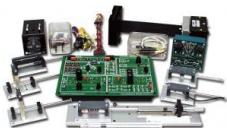
The measurements package is an instrumentation module with signal conditioning circuitry and includes a wheatstone bridge, oscillator, operational amplifier, discriminator and power amplifier.
