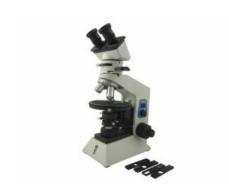
This trinocular microscope is specially designed for research in the field of geology, petrography, mineralogy and medical science.
